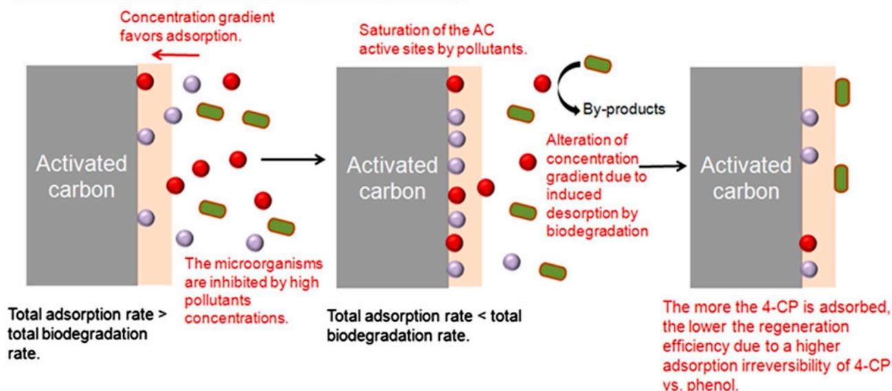
Fig. 1. Schematic illustration of the two approaches of bioregeneration of GAC loaded with phenol and 4-CP.
