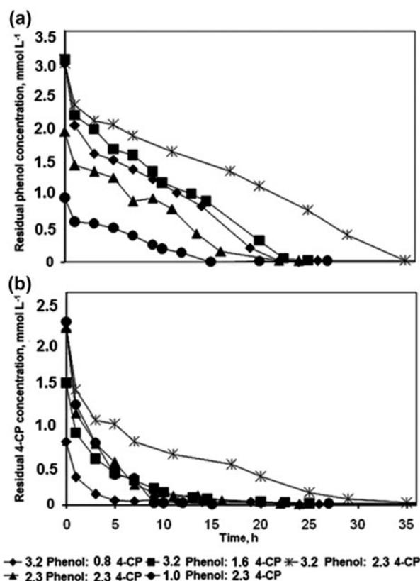
Fig. 2. Time courses of the (a) residual phenol and (b) 4-CP concentrations at various initial concentrations of phenol and 4-CP during the simultaneous adsorption and biodegradation processes.
