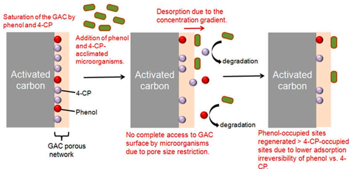
**Simultaneous adsorption and biodegradation (one-step)**
