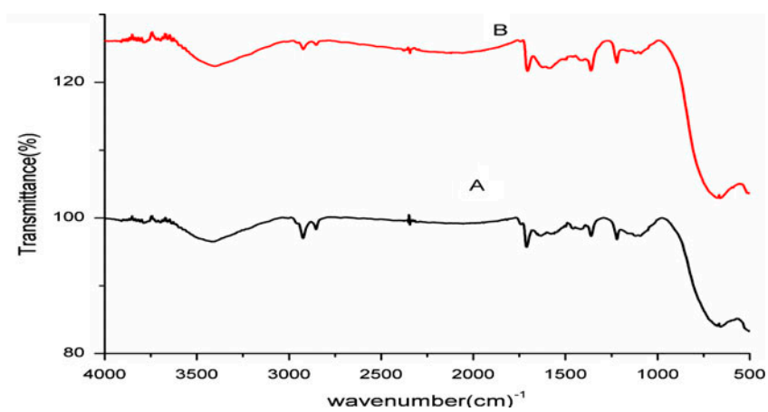
Fig. 4. FT-IR spectra of \text{TiO}_2/\text{AC} nanocomposite (A) after degradation and (B) before degradation of dye.
