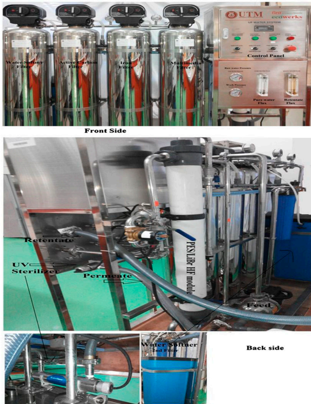
Fig. 1. The front and back view of the UF system with HF membrane module.
