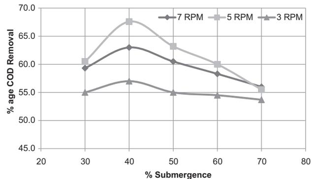
Fig. 4. COD removal efficiencies at different RPM and submergences.
