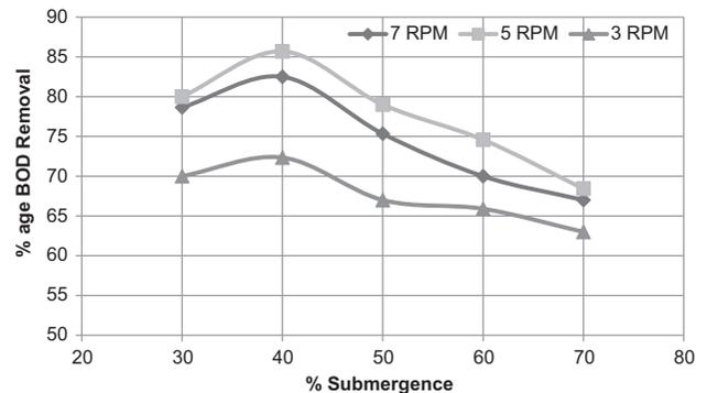
Fig. 3. BOD removal efficiencies at different RPM and submergences.
