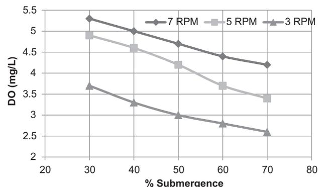
Fig. 2. DO concentration at different RPM and submergences.
