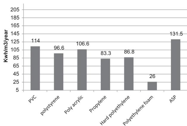
Fig. 6. Energy consumption for different RBC disc materials ASP.
