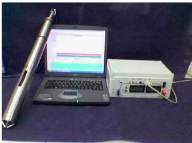
Fig. 1. The multi-parameter sensors system (Watertool II).
