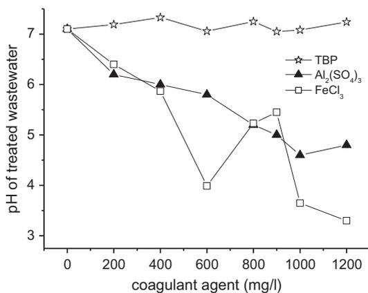
Fig. 3. Effect of coagulant agents on treated wastewater pH.
