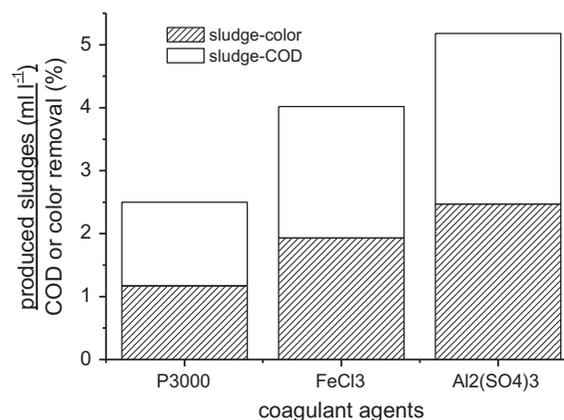
Fig. 5. Ratios between the amount of sludge produced and COD or color removal.
