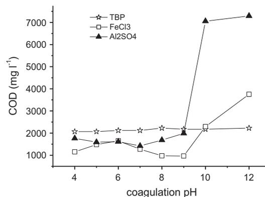
Fig. 2. Effect of coagulation pH on COD removal (coagulant =  $400 \text{ mg l}^{-1}$ ).
