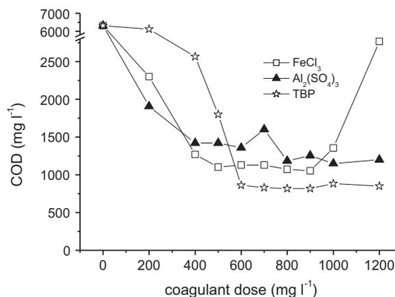
Fig. 4. Effect of coagulant dosage on COD removal.
