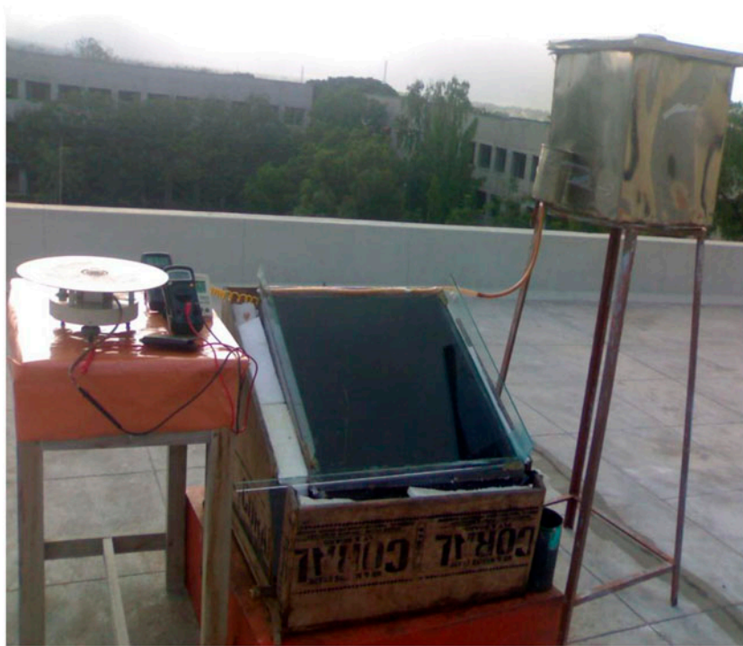
Fig. 2. Pictorial view of single-slope solar still.
