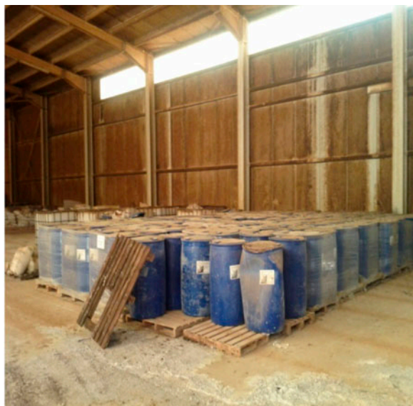
Fig. 5. Chemical storage department at Tajoura desalination plant: (a) acid is spilled in the floor and (b) dust is all over the place.
