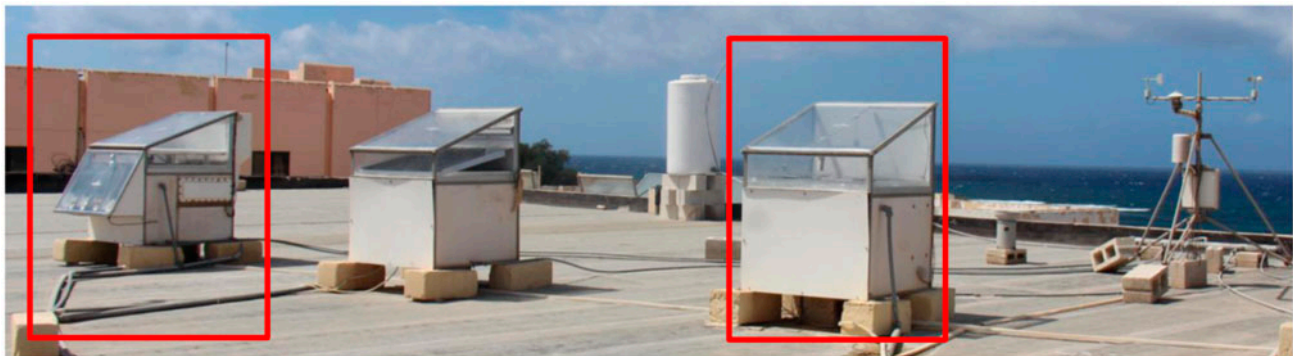
Fig. 12. Solar still set-up on roof (only two out of the three units shown are described in this paper).
