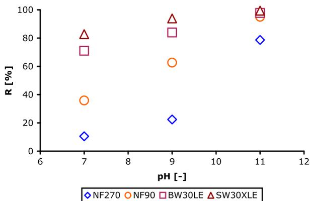
Fig. 5. Maximum boron rejection ( $R$ ) values gathered on selected membranes at various pH values, feeding a test solution containing about 50 mg/L of boron.
