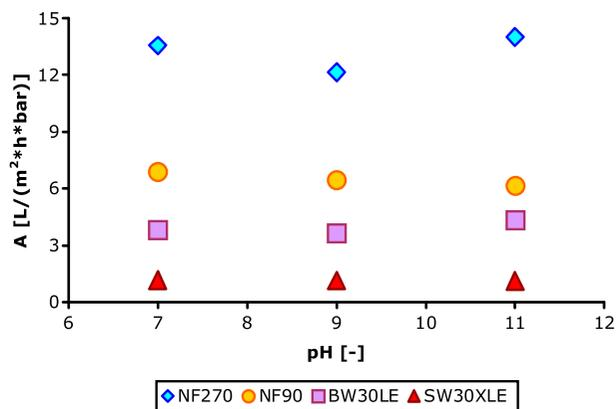
Fig. 4. Mean water permeability ( $A$ ) values gathered on selected membranes at various pH values, feeding a test solution containing about 50 mg/L of boron.
