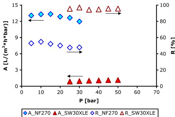
Fig. 2. Example of screening experiments. Water permeability (*A*) values and conductivity rejection (*R*) values were collected, respectively, for the SW30XLE and the NF270 membranes, both tested with water at pH of 11.
