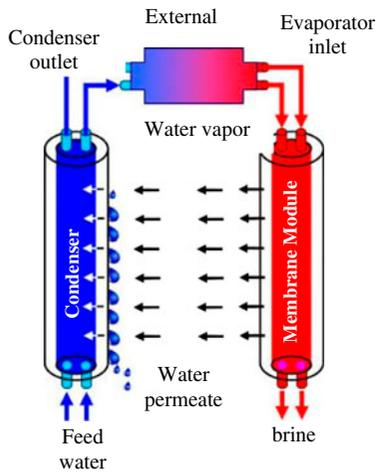
Fig. 12. Schematic layout of one element of the Memstill process.
