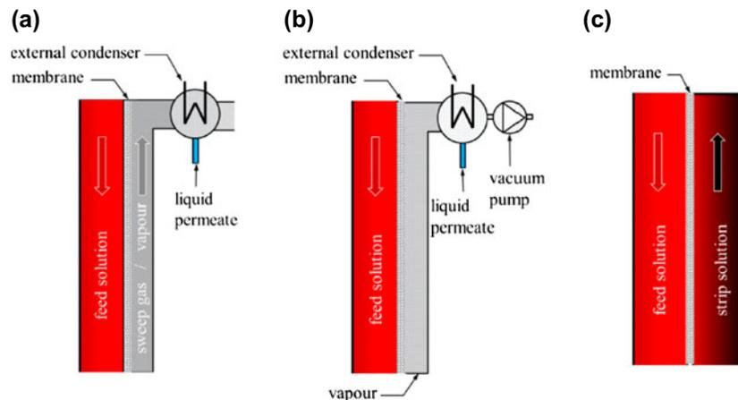
Fig. 4. MD configurations driven by approaches other than a temperature difference: (a) SGMD, (b) VMD, and (c) OMD.
