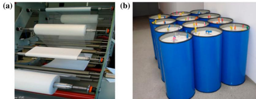
Fig. 6. (a) Spiral-wound winding machine and (b) Picture of the modules.
