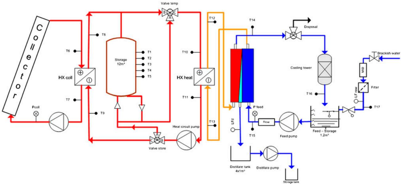
Fig. 9. Schema of the Namibia plant.
