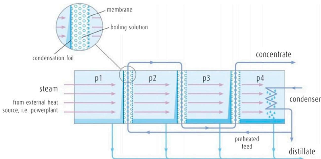
Fig. 18. Basic principles of memsys V-ME-MD [40].
