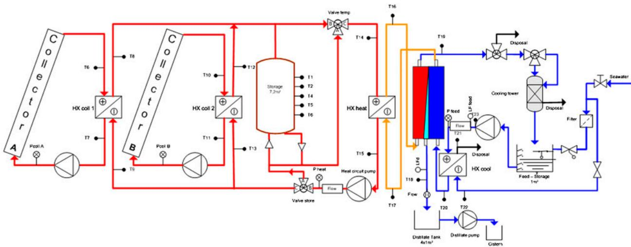
Fig. 10. Schema of the Gran Canary plant.
