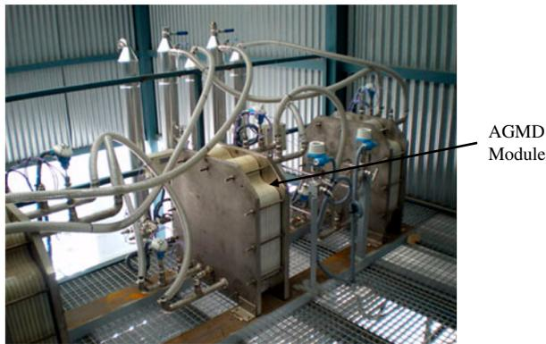
Fig. 16. Scarab membranes for distillation in the experimental installation built at PSA-CIEMAT (Almería, Spain) [39].
