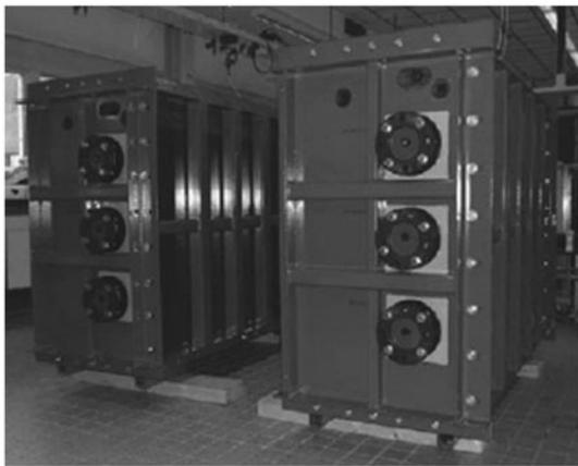
Fig. 13. Membrane modules for pilot plant.
