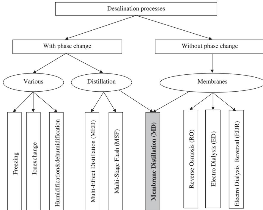
Fig. 1. Classification of water desalination technologies.
