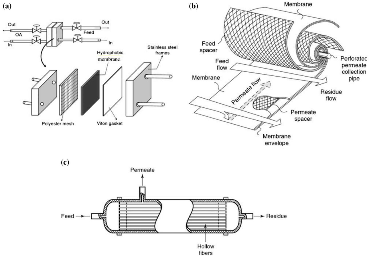
Fig. 5. Schematic illustration of the different basic module design principles: (a) plate-and-frame module, (b) spiral-wound module, and (c) shell and tube.
