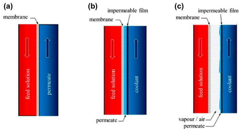
Fig. 3. MD configurations driven by a temperature difference: (a) DCMD, (b) PGMD, and (c) AGMD.
