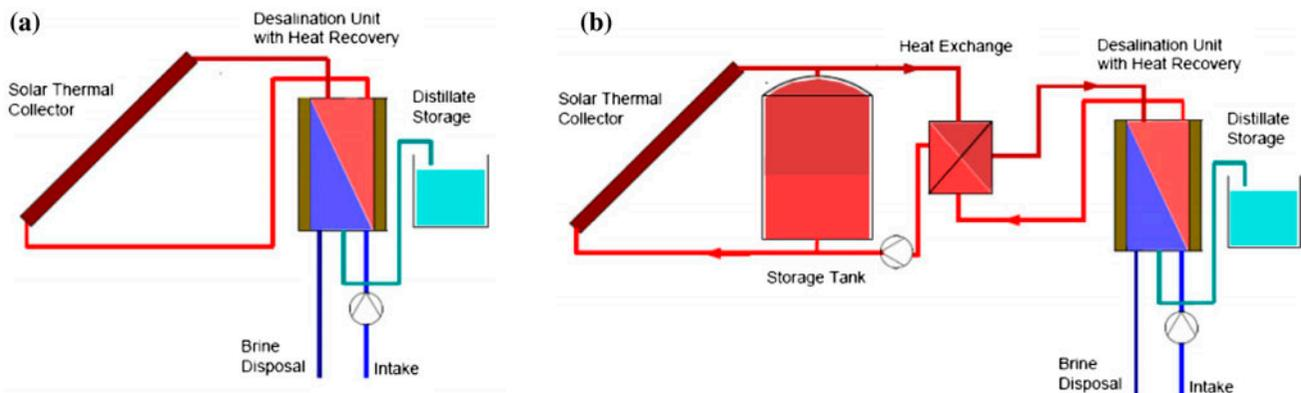
Fig. 7. Two different system configuration: (a) compact system and (b) two-loop system [22].
