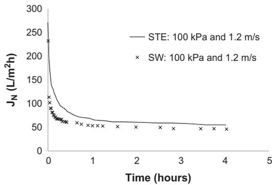
Fig. 1. Permeate flux decline vs. time with a hollow-fiber diameter of 1.5 mm.
