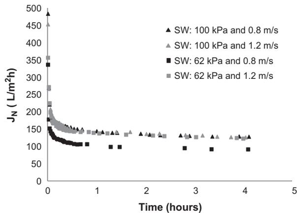
Fig. 7. Permeate flux decline vs. time with the membrane of 0.8 mm of diameter.
