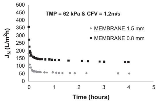
Fig. 5. Permeate flux decline vs. time with SW at 62 kPa and 1.2 m/s.
