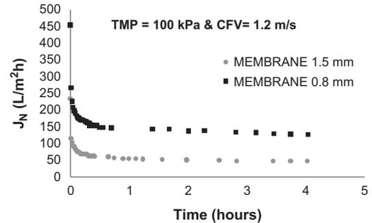
Fig. 6. Permeate flux decline vs. time with SW at 100 kPa and 1.2 m/s.
