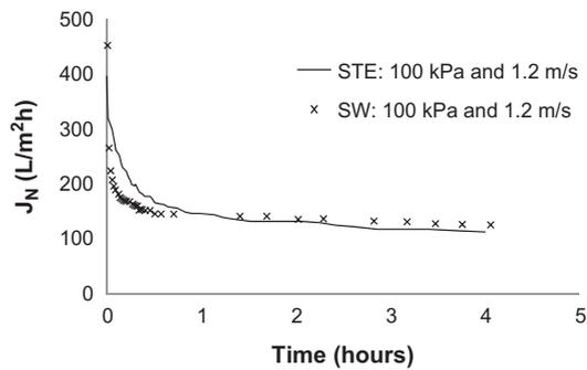
Fig. 2. Permeate flux decline vs. time with a hollow-fiber diameter of 0.8 mm.
