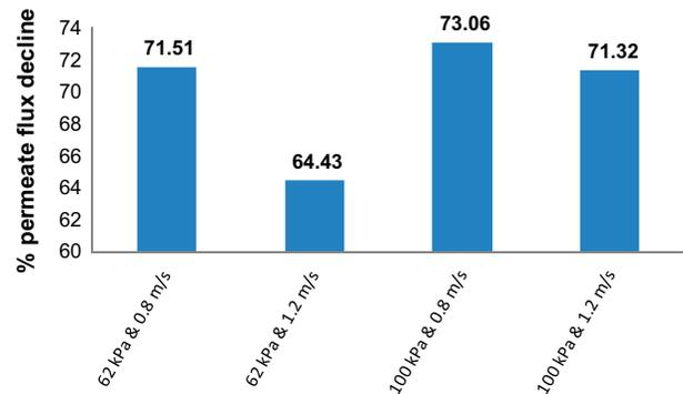
Fig. 8. Percentage of permeate flux decline for each operating condition.
