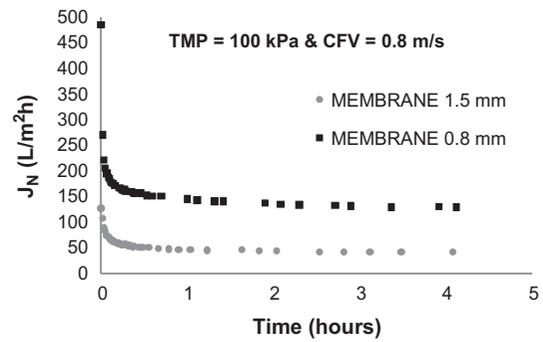
Fig. 4. Permeate flux decline vs. time with SW at 100 kPa and 0.8 m/s.
