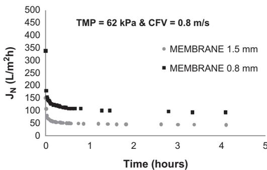
Fig. 3. Permeate flux decline vs. time with SW at 62 kPa and 0.8 m/s.
