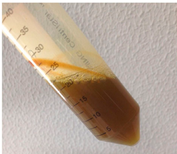
Fig. 1. Sample of spent pickling liquor.
