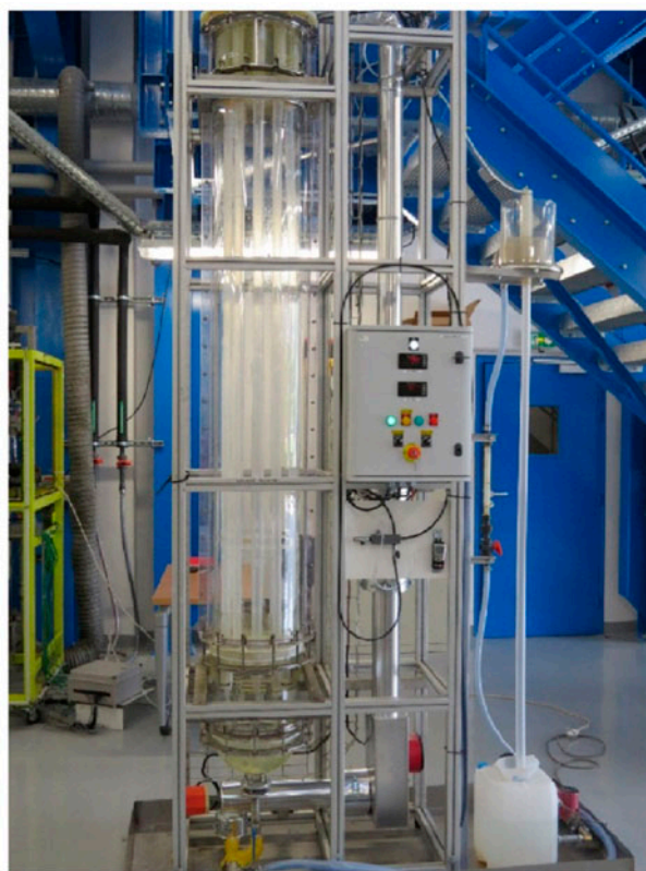
Fig. 7. Ageing and wetting test rig of polymer tubes.
