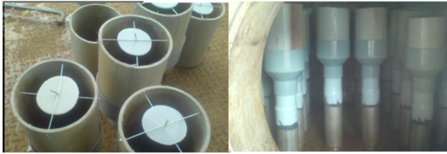
Fig. 12. Increased spouts pipe height with cone expander at spout tip inside chamber.
