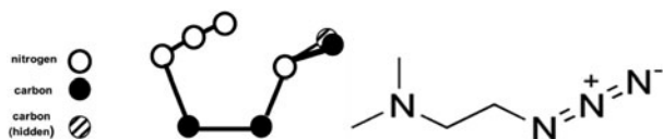
Fig. 1. Semi-ring structure (left) and linear structure (right) of DMAZ molecule [6].
