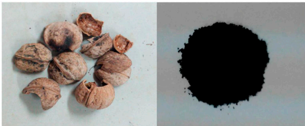
Fig. 2. A photo of walnut shell (from gardens of Touiserkan, Iran)-left side; and the resultant activated carbon-right side.
