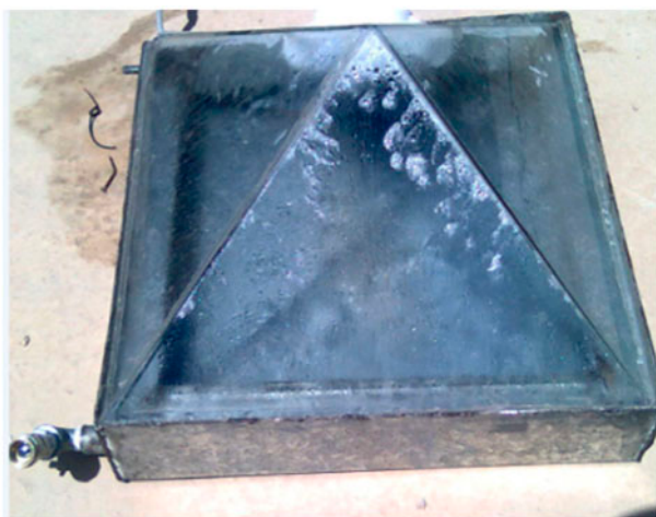
Fig. 1. Photograph of pyramid-shaped solar still.
