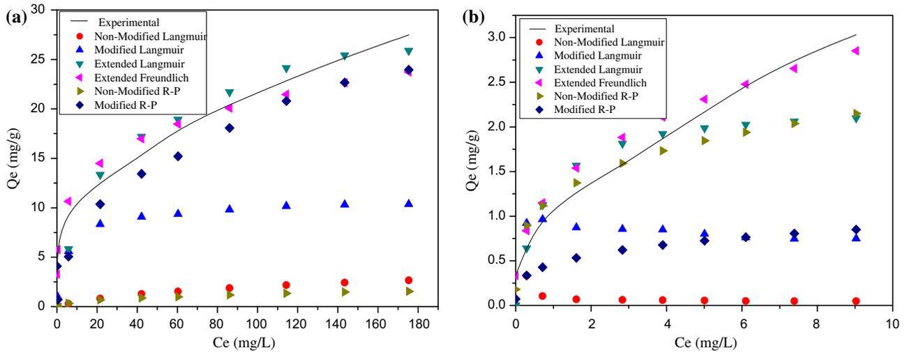
Fig. 12. (a) Comparison of binary component isotherm model for phenol and (b) comparison of binary component isotherm model for cyanide.
