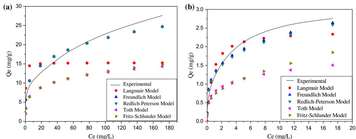
Fig. 11. (a) Comparison of monocomponent isotherm model for phenol and (b) comparison of monocomponent isotherm model for cyanide.
