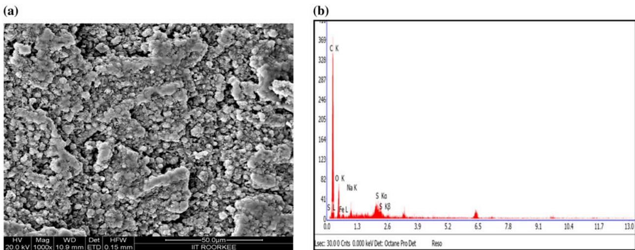
Fig. 4. (a) SEM image of CSAC after simultaneous biosorption and bioaccumulation and (b) EDX analysis of CSAC after simultaneous biosorption and bioaccumulation.
