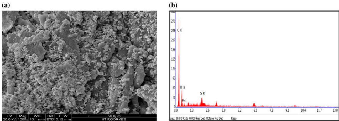
Fig. 3. (a) SEM image of CSAC after immobilization of micro-organism and (b) EDX analysis of CSAC after immobilization of micro-organism.
