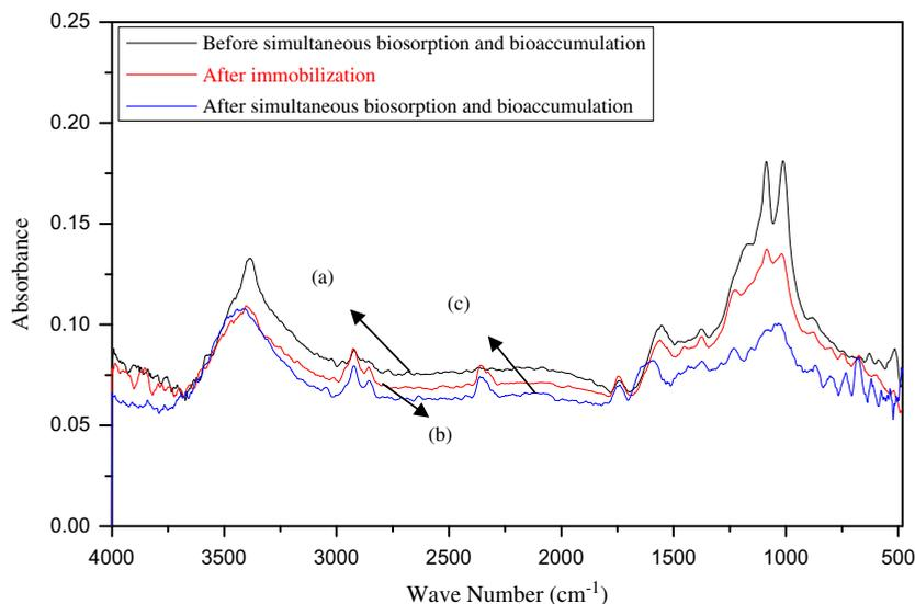
Fig. 5. FTIR spectrum of CSAC: (a) before simultaneous biosorption and bioaccumulation, (b) after immobilization of co-culture and (c) after simultaneous biosorption and bioaccumulation of phenol and cyanide.
