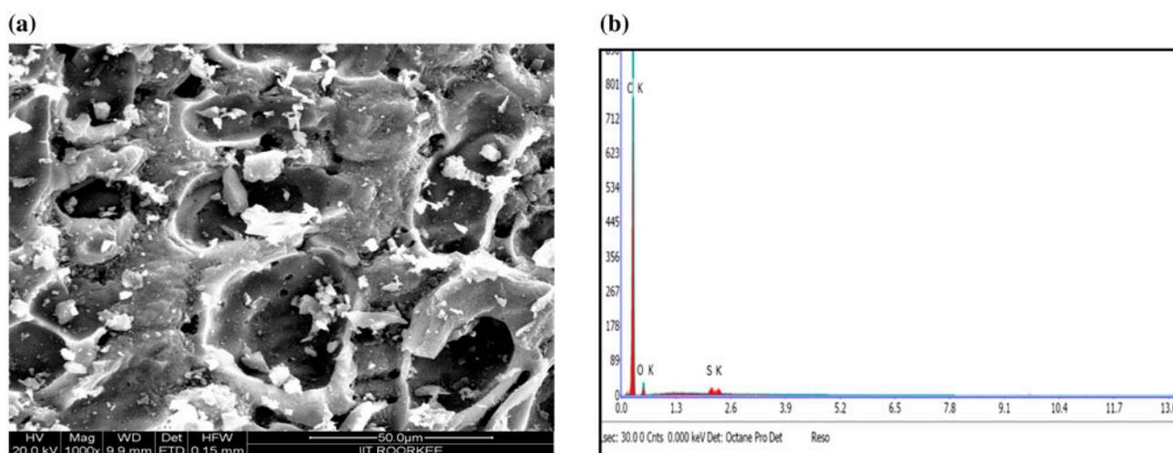
Fig. 2. (a) SEM image of CSAC before biosorption and (b) EDX analysis of CSAC before biosorption.
