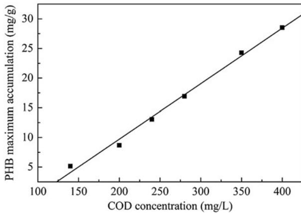
Fig. 5. The linear relationship between COD concentrations and maximum net PHB accumulation.
