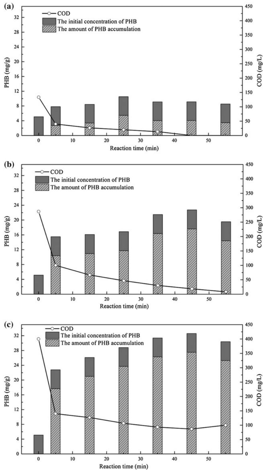
Fig. 4. Changes in PHB and COD profiles at different influent COD concentrations: (a) COD concentration: 133.33 mg/L, (b) COD concentration: 266.67 mg/L, and (c) COD concentration: 400.00 mg/L.
