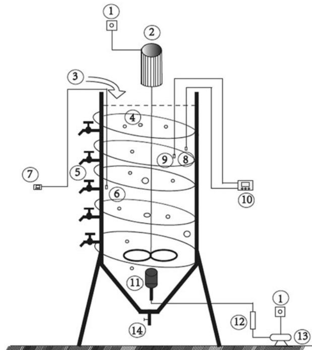
Fig. 1. Schematic diagram of (a) SBR.
