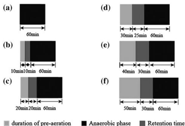
Fig. 2. Operating strategies with different pre-aeration times (the fixed pre-aeration flux is 35 L/h).
