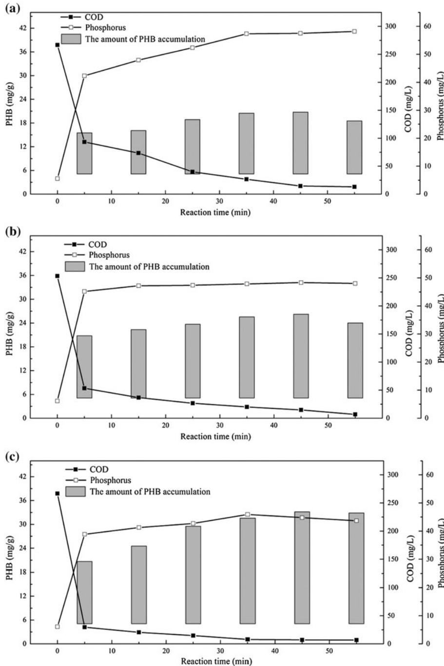
Fig. 7. Changes in PHB, TP, and COD profiles at different pre-aeration time: (a) without pre-aeration, (b) pre-aeration time of 10 min, (c) pre-aeration time of 20 min, (d) pre-aeration time of 30 min, (e) pre-aeration time of 40 min, and (f) pre-aeration time of 50 min.
