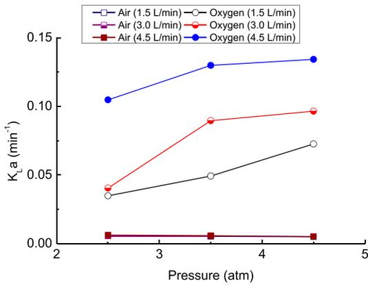
Fig. 4. Volumetric oxygen transfer coefficient for each operating condition.
