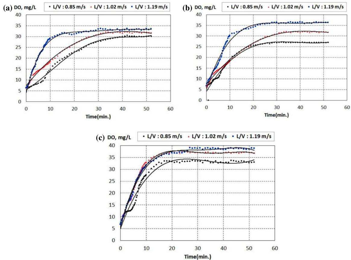
Fig. 2. Transient DO concentration profiles at various oxygen supply velocity: (a) 1.27 m/s, (b) 2.55 m/s, (c) 3.82 m/s ( $L/V$  refers to liquid velocity).
