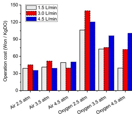
Fig. 6. Operation cost by each operating condition.
