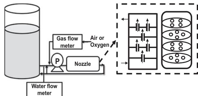
Fig. 1. Schematic diagram of the bubble generator.
