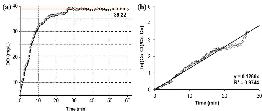
Fig. 3. (a) DO variation with time at gas velocity 3.82 m/s and liquid velocity 1.19 m/s and (b) a result of application for volumetric oxygen transfer model.
