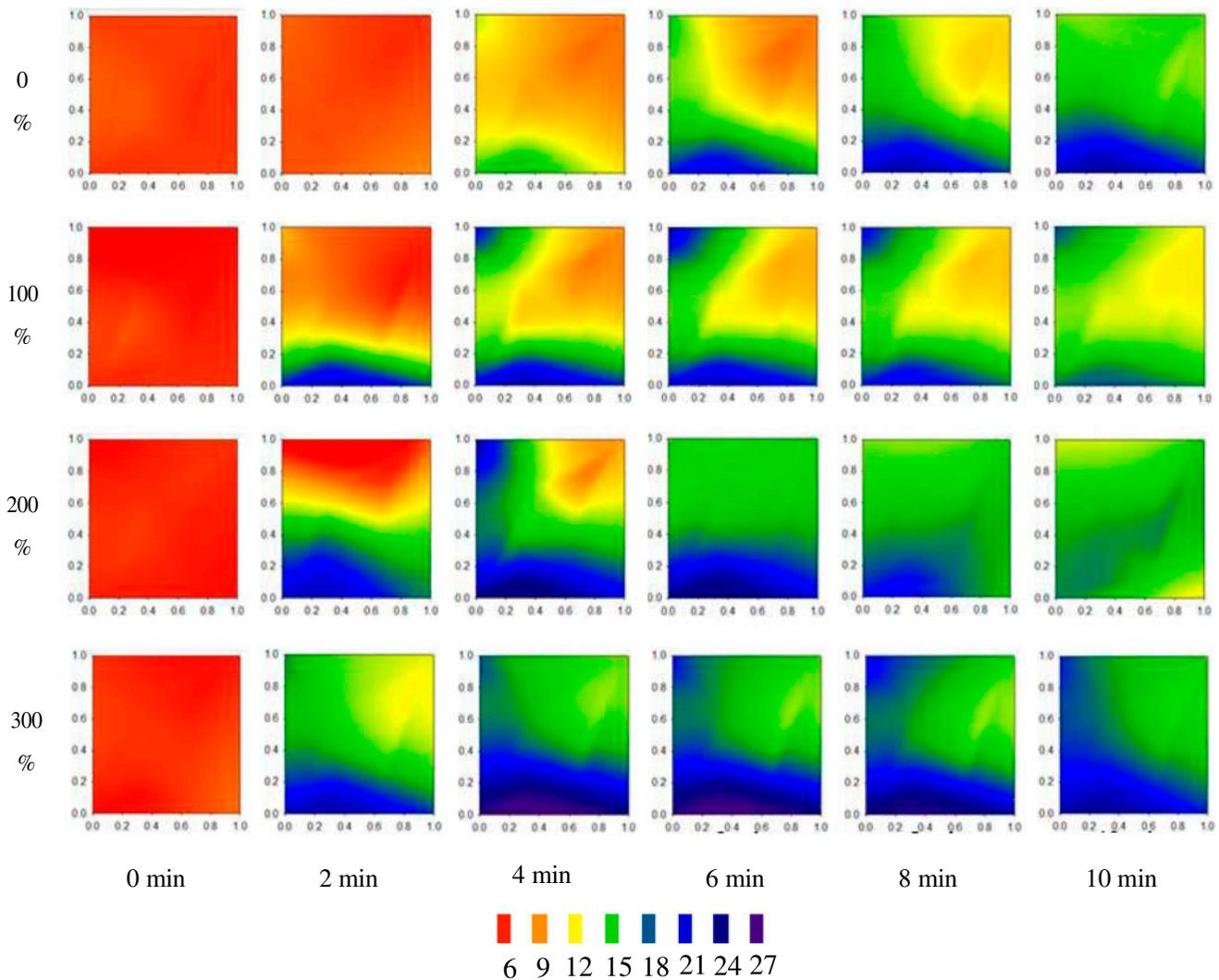
Fig. 5. Time variation of DO concentration by circulation rate and depth (x axis: width (m) and y axis: height (m)).
