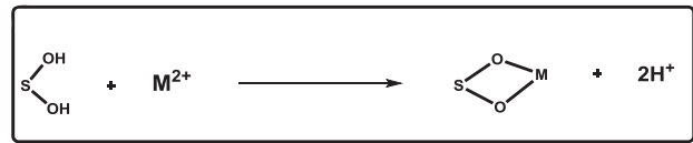
Fig. 5. Schematic representation of M 2+ ion coordinating with adjacent hydroxyl groups on the surface of the adsorbent.
