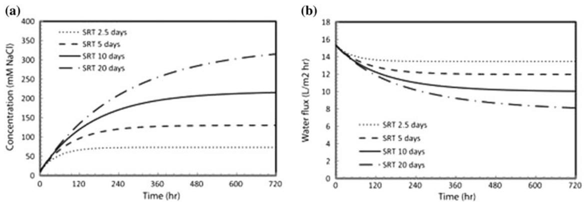
Fig. 6. Relationships between theoretical salt accumulation (a) model in bioreactor and water flux (b) under different SRT [54].
