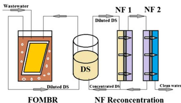
Fig. 9. Schematized FOMBR system with NF reconcentration process.
