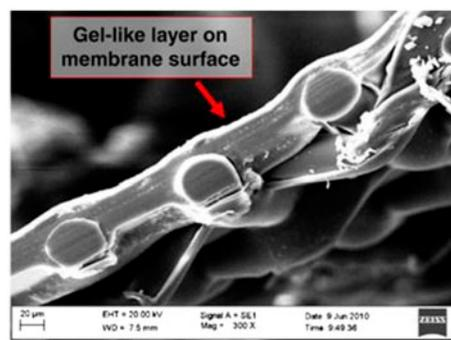
Fig. 14. SEM image of the cross section of the used membrane together with the thin gel-like layer [137].
