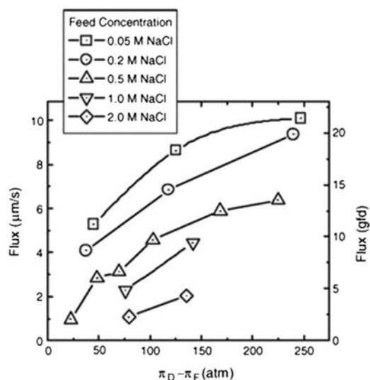
Fig. 8. Flux data for a variety of feed solution [NaCl] concentrations. The water flux is presented as a function of the difference in bulk osmotic pressures of the draw and feed solutions. Experimental conditions: crossflow velocity and temperature of both feed and DS of 30 cm/s and 50 °C, respectively [14].
