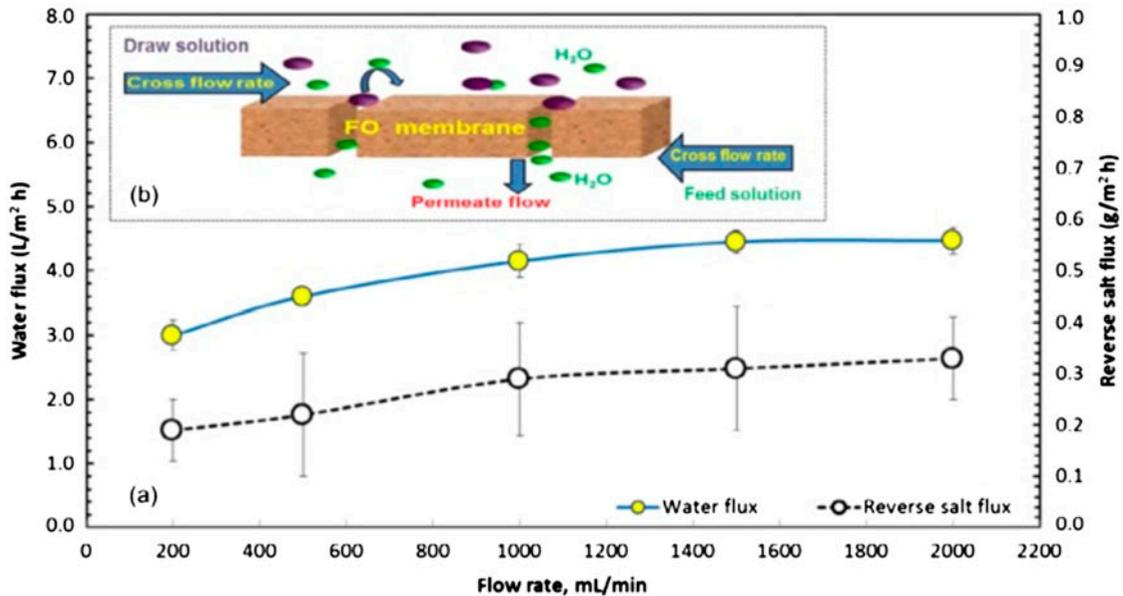
Fig. 11. Water flux and reverse salt flux as a function of draw solution flow rates (FS: DI water; DS: 1 M EDTA-2Na; CTA-NW FO membrane in AL-FS mode) (figure obtained from Ref. [128] with copyright permission).
