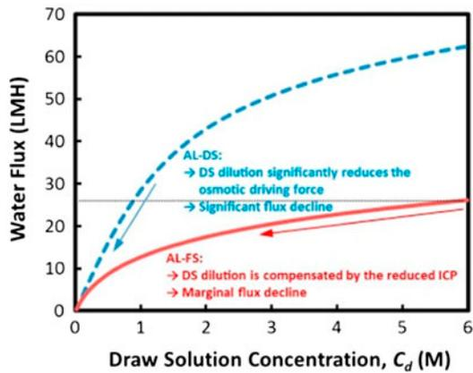
Fig. 10. Fouling effect of different DS concentrations (figure obtained from Ref. [128] with copyright permission).
