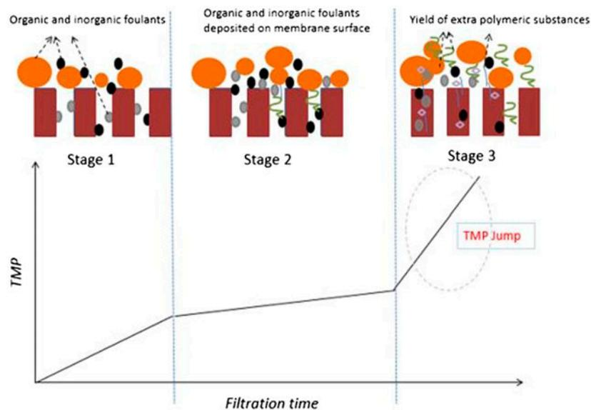
Fig. 12. Schematic illustration of the occurrence of TMP jump.
