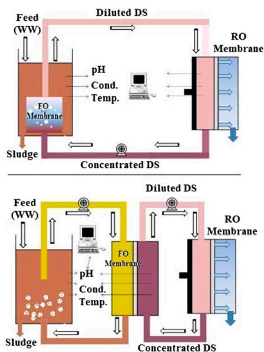
Fig. 5. Submerged (above) and side-stream (below) configuration in FOMBR.
