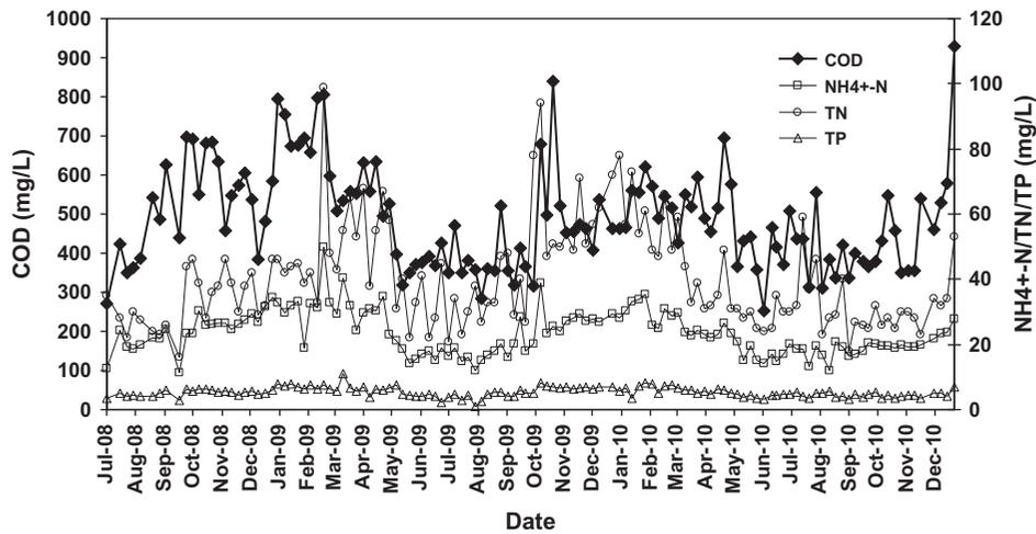
Fig. 1. Change of influent COD,  $\text{NH}_4^+\text{-N}$ , TN and TP over 2008–2010.
