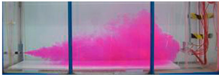
Fig. 2. Cold water jet instantaneous image for \Delta T_0 = -3^\circ\text{C} .
