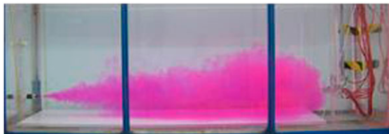
Fig. 4. Cold water jet instantaneous image for \Delta T_0 = -7^\circ\text{C} .
