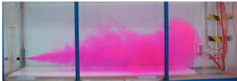
Fig. 3. Cold water jet instantaneous image for \Delta T_0 = -5^\circ\text{C} .
