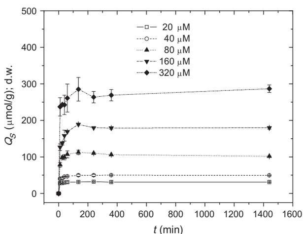
Fig. 1. Effect of contact time and concentration of CdCl<sub>2</sub> on Cd adsorption by dried biomass of the freshwater moss *V. dubyana* (0.5 g/l; d.w.) under initial conditions of pH 4.0 and 25°C.
