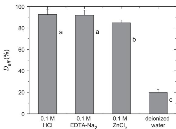
Fig. 6. Efficiency of Cd desorption from dried biomass of the freshwater moss *V. dubyana* (0.5 g/l; d.w.) after 2 h batch desorption. Adsorption experiment: 2 h in a 320  $\mu$ M  $CdCl_2$  solution at initial pH 4.0 and 25°C. Means with the same letter in columns are not significantly different at the  $p = 0.05$  level based on the multiple range test.
