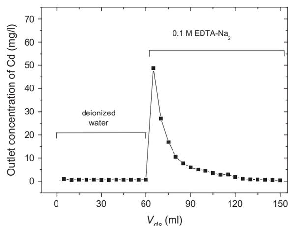
Fig. 7. Desorption of Cd from dried biomass of the freshwater moss *V. dubyana* (0.05 g; d.w.) by a two-step desorption with deionized water and 0.1 M EDTA- $Na_2$  in a packed bed column system.
