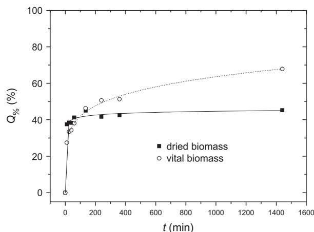
Fig. 2. Kinetics of Cd uptake by dried and vital *V. dubyana* moss biomass (0.5 g/l; d.w.) from a 320  $\mu\text{M}$  CdCl<sub>2</sub> solution under initial conditions of pH 4.0 and 25°C.
