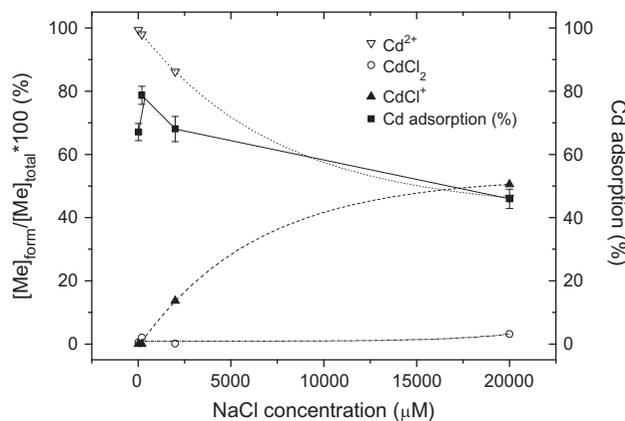
Fig. 4. Effect of NaCl concentration on Cd speciation in solution and Cd adsorption by dried biomass of the freshwater moss *V. dubyana* (0.5 g/l; d.w.) after 2 h of exposure in a solution containing 20  $\mu\text{M}$   $\text{CdCl}_2$  at initial  $\text{pH}$  4.0 and 25°C.
