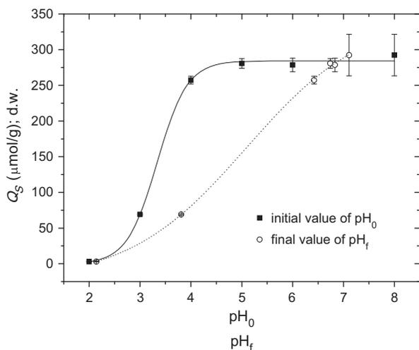
Fig. 3. Effect of  $\text{pH}$  on Cd adsorption by dried biomass of the freshwater moss *V. dubyana* (0.5 g/l; d.w.) after 2 h of exposure in a solution containing 320  $\mu\text{M}$   $\text{CdCl}_2$ .
