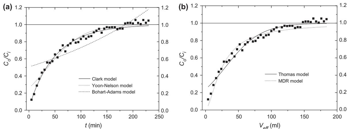
Fig. 5. Kinetics of Cd adsorption by dried biomass of the freshwater moss *V. dubyana* (0.05 g; d.w.) in a packed bed column system described as  $C_0/C_i$  vs.  $t$  (a) or  $C_0/C_i$  vs.  $V_{\text{eff}}$  dependence (b) at a flow rate of 0.80 ml/min and 25°C. The initial conditions were 36 mg/l  $\text{CdCl}_2$  and pH 6.0.
