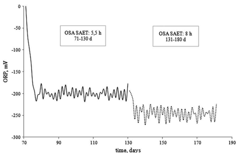
Fig. 2. Evolution of ORP in the anaerobic tank during the OSA stages.
