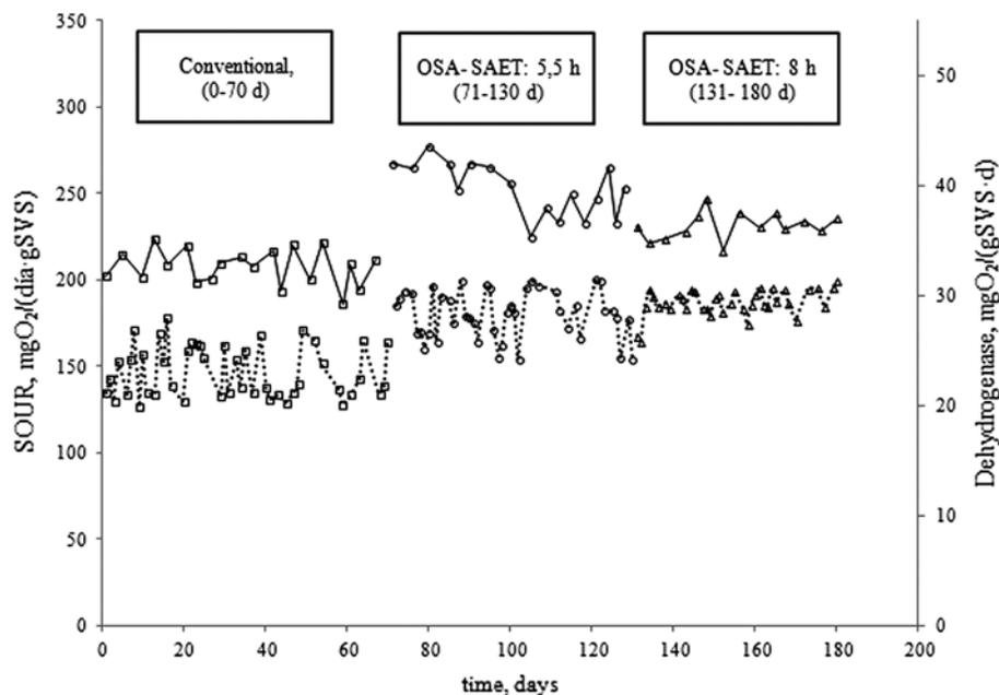
Fig. 3. Biomass activity measured SOUR (dotted line) and DHA tests (solid line) during study.
