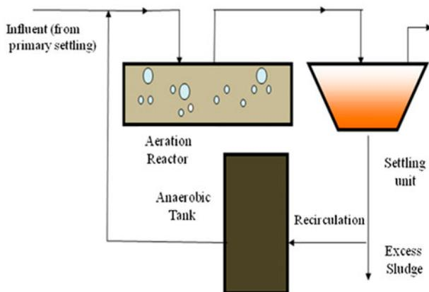
Fig. 1. Oxic-settling-anaerobic (OSA) process.
