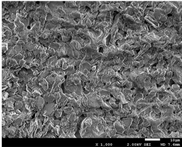
Fig. 4. Picture by SEM showing the microstructure of the  $\text{Al}_2\text{O}_3\text{-TiO}_2$  membrane body. Pore sizes are 1–2  $\mu\text{m}$ , approximately.
