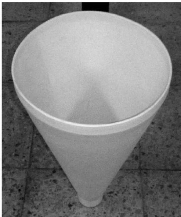
Fig. 1. Ceramic macromembrane made of  $\text{Al}_2\text{O}_3\text{-TiO}_2$ : maximum inner diameter, 400 mm; minimum inner diameter, 40 mm; height, 500 mm; thickness, 8 mm.
