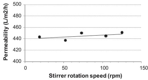
Fig. 6. Effect of stirring in the performance of the macromembrane. Operating conditions: inlet temperature = 18°C; inlet flowrate = 890 L/h; pressure = 1.5 bar; duration of each measure = 10 min.
