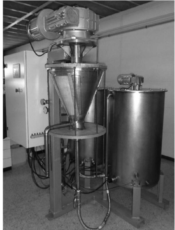
Fig. 3. Pilot plant for testing macromembrane performance.
