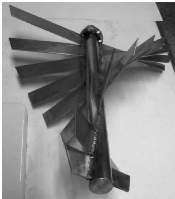
Fig. 2. Experimental stirrer used in pilot tests.
