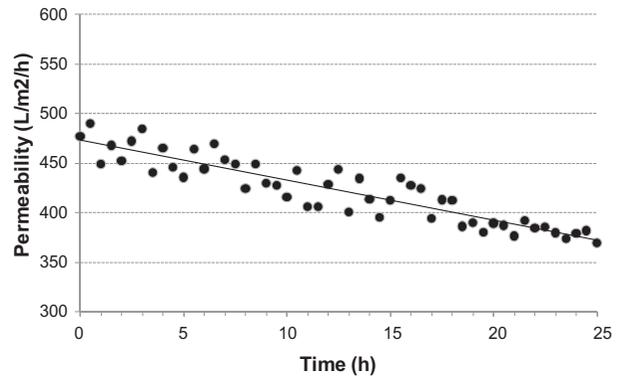
Fig. 7. Performance of the macromembrane in the pilot plant. Permeability vs. time at constant operating conditions: inlet temperature = 20°C; inlet flowrate = 890 L/h; pressure = 1.5 bar; no stirring.
