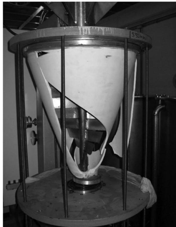
Fig. 5. Picture of the macromembrane broken at 2.5 bars. The stirrer can be seen in the interior of the macromembrane.
