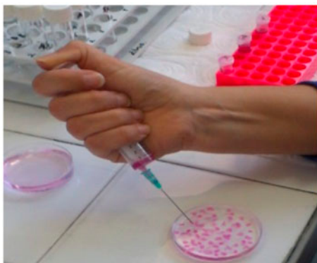
Fig. 1. Preparation of the exoPS gels by dropping i.e. 0.2% exoPS into 0.2% \text{CaCl}_2 solution.
