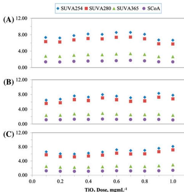
Fig. 1. Specific UV-vis parameters of HA following adsorption onto sole  $\text{TiO}_2$  (A),  $\text{TiO}_2$  and Kt (B), and  $\text{TiO}_2$  and Mt (C).
