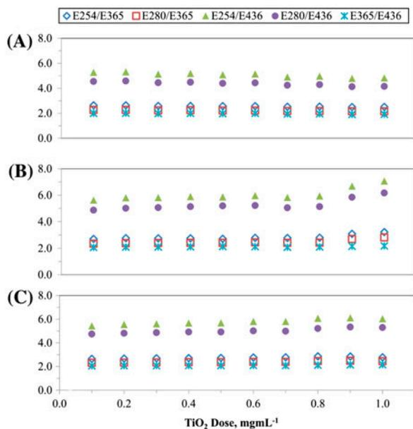
Fig. 3. Fractional UV-vis parameters of HA following adsorption onto sole TiO<sub>2</sub> (A), TiO<sub>2</sub> and Kt (B), TiO<sub>2</sub> and Mt (C).
