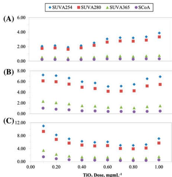
Fig. 2. Specific UV–vis parameters of HA following adsorption onto sole  $\text{TiO}_2$  (A),  $\text{TiO}_2$  and Kt (B), and  $\text{TiO}_2$  and Mt (C) in the presence  $\text{Ca}^{2+}$  ions.
