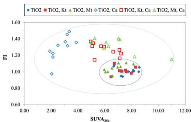
Fig. 8. Correlation of SUVA<sub>254</sub> with FI in the absence and presence of Ca<sup>2+</sup> ions.
