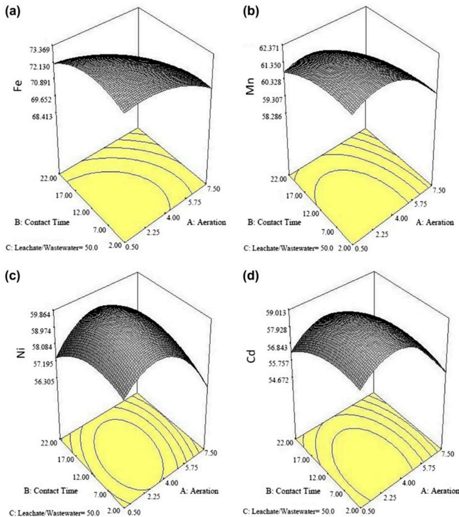
Fig. 3. The 3-D surface plots of (a) Fe, and (b) Mn, (c) Ni, and (d) Cd removal in PZ-SBR.
