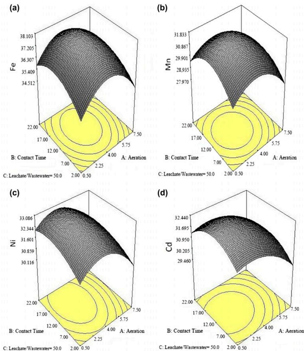
Fig. 2. The 3-D surface plots of (a) Fe, and (b) Mn, (c) Ni, and (d) Cd removal in normal-SBR.
