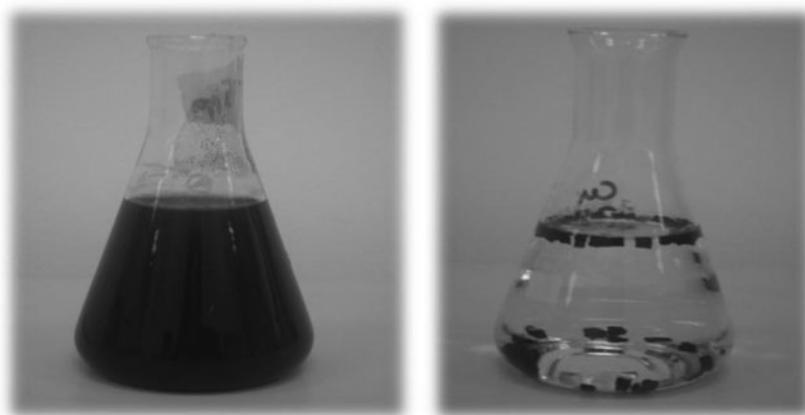
Fig. 6. Comparison between a sample solution with biochar and HBC-RH as sorbent (Left: Biochar in solution; Right: HBC-RH in solution).
