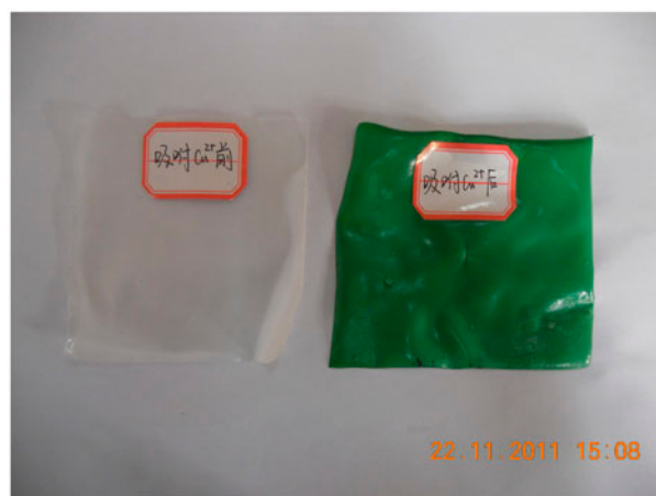
Fig. 8. The surface color of the original sample D (left) and the adsorbed sample D (right), respectively.
