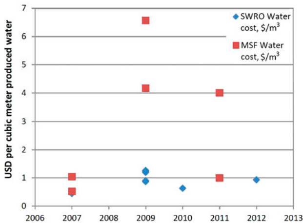
Fig. 7a. Cost of water production with MSF and SWRO in Arabian Gulf waters, 2007–2012 [15].
