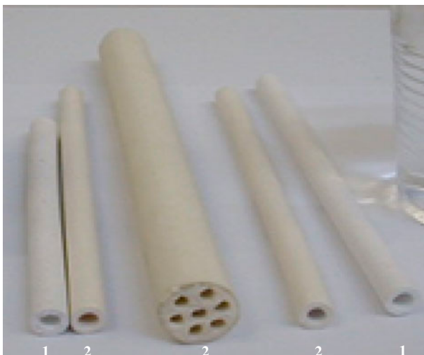
Fig. 6. Image of tubular membranes supports prepared from two different kaolin types, 1: DD2 kaolin type, 2: another kaolin type.
