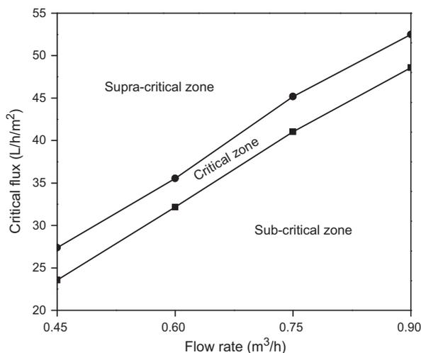
Fig. 3. Variations of CF with aeration flow rate.
