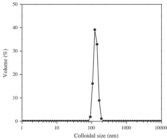
Fig. 7. Particle size distribution of colloids in the supernatant.
