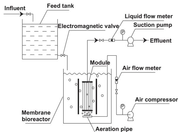
Fig. 1. Schematic of the experimental system setup.
