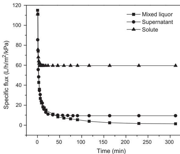
Fig. 6. Variations of specific flux with time during filtration of various sludge fractions.
