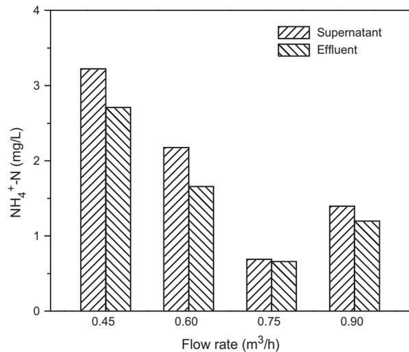
Fig. 9. Supernatant NH<sub>4</sub><sup>+</sup>-N and effluent NH<sub>4</sub><sup>+</sup>-N at different flow rates.
