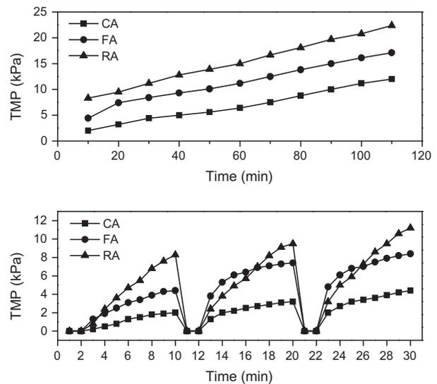
Fig. 2. Changes in TMP with time at different aeration modes (aeration intensity = 0.7 m<sup>3</sup>/h, flux = 28.32 L/(h m<sup>2</sup>)).
