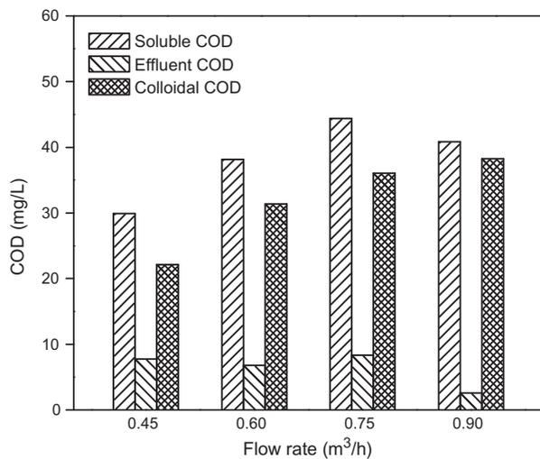
Fig. 8. Concentrations of soluble COD, effluent COD, and colloidal COD at different flow rates.
