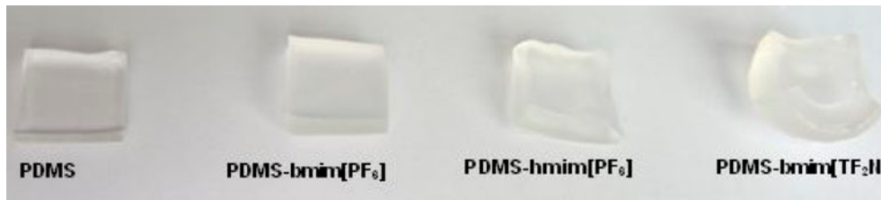
Fig. 6. The membranes after reaching sorption equilibrium in BuOH.
