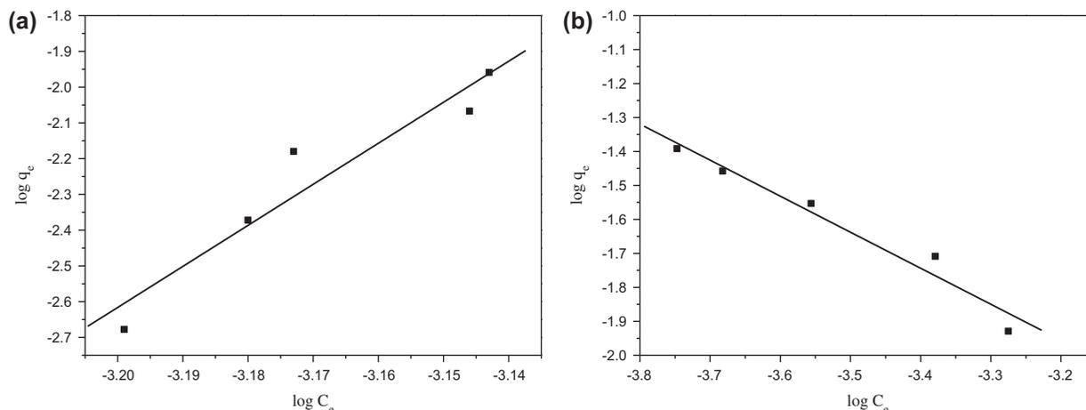
Fig. 9. Freundlich plot for the sorption of Pb(II) on (a) SCB and (b) BP at constant temperature.
