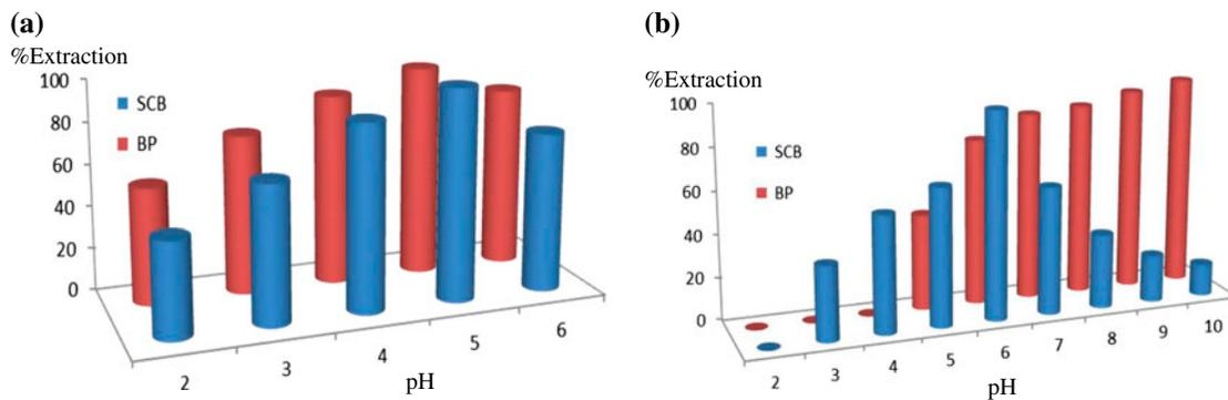
Fig. 5. Percentage extraction of (a) Pb(II) and (b) Na(I) as a function of pH using SCB and BP.
