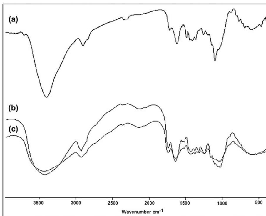
Fig. 2B. FT-IR spectra of (a) BP, (b) BP-Pb(II), and (c) BP-Na(I) phases.
