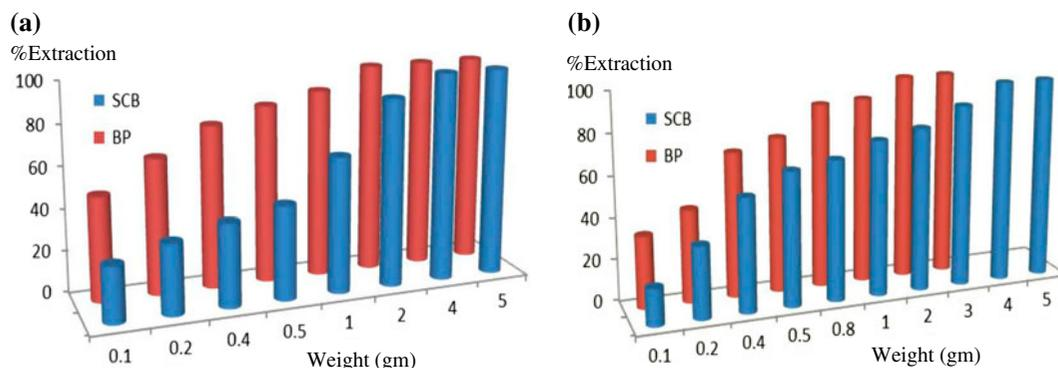
Fig. 6. Effect of SCB and BP weight on % extraction of (a) Pb(II) and (b) Na(I).
