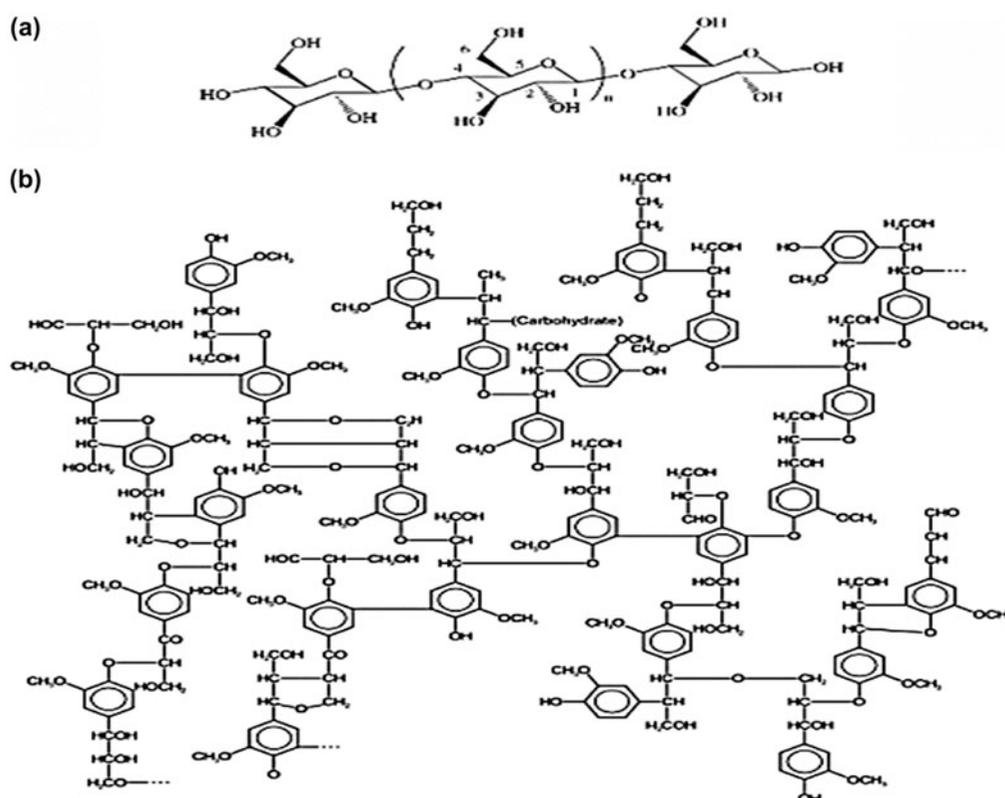
Fig. 1. Chemical structure of (a) cellulose and (b) lignin in SCB and BP molecules.
