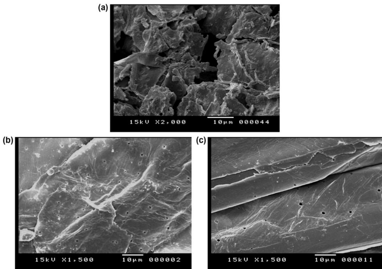
Fig. 4A. SEM images of (a) SCB (b) SCB with Pb(II), and (c) SCB with Na(I).
