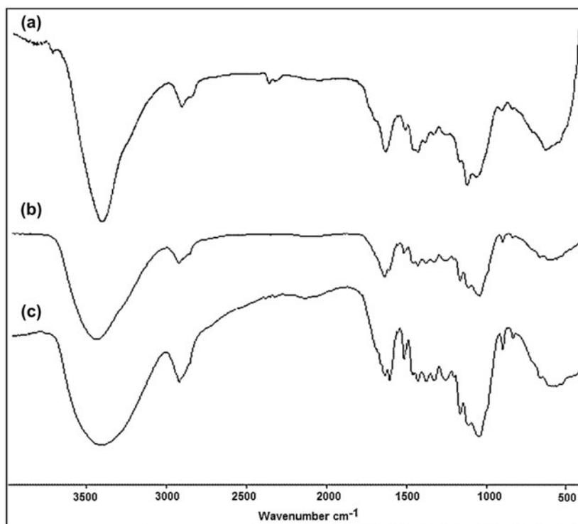
Fig. 2A. FT-IR spectra of (a) SCB, (b) SCB-Pb(II), and (c) SCB-Na(I) phases.
