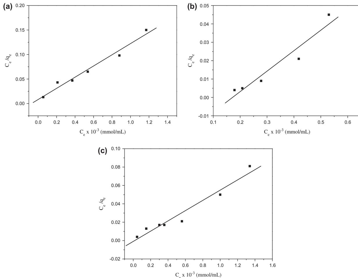
Fig. 10. Langmuir plot for the sorption of (a) Na on SCB, (b) Pb(II) and (c) Na(I) on BP at constant temperature.
