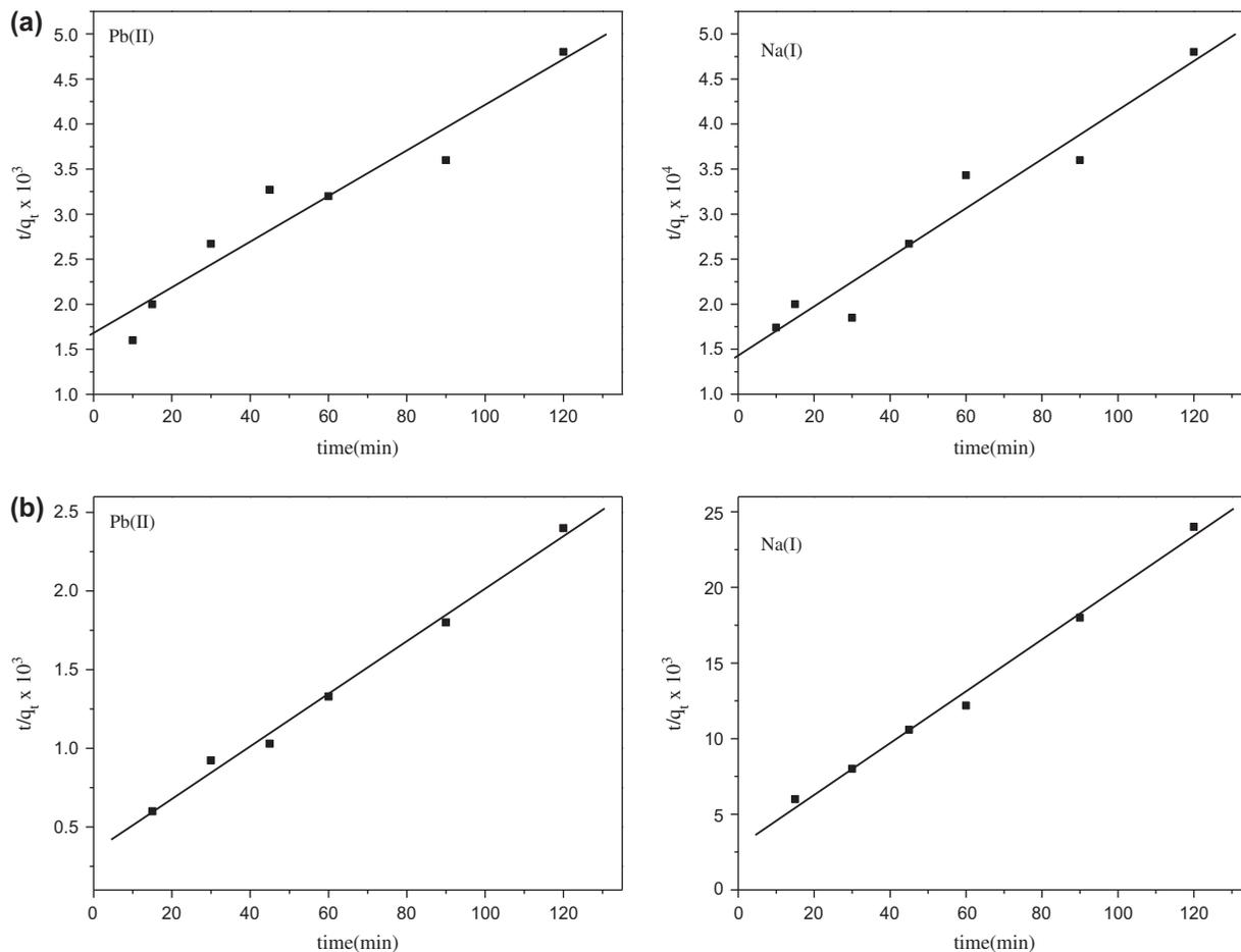
Fig. 8. Pseudo-second-order kinetic plots for the sorption of Pb(II) and Na(I) on: (a) SCB and (b) BP.
