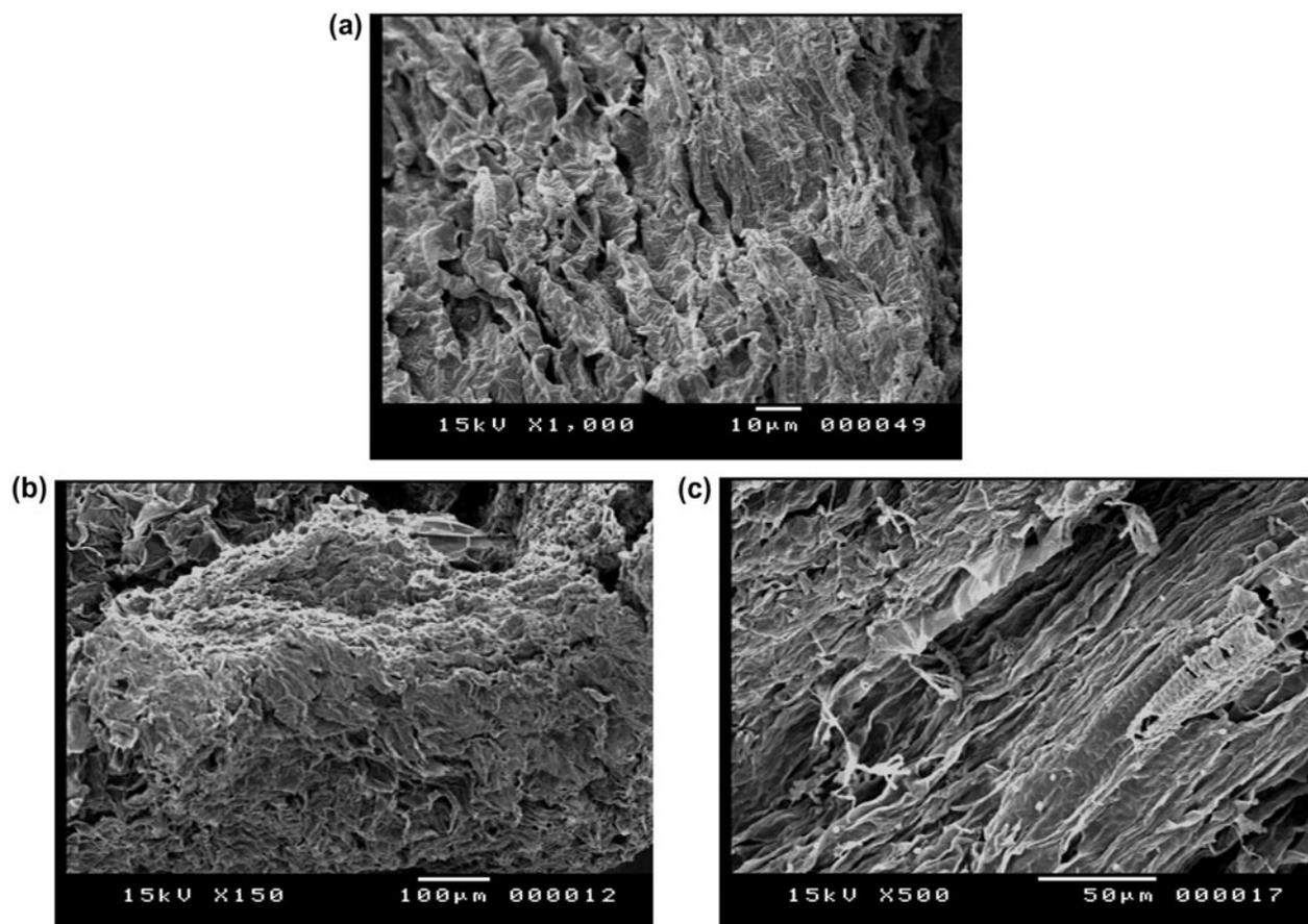
Fig. 4B. SEM images of (a) BP (b) BP with Pb(II), and (c) BP with Na(I).
