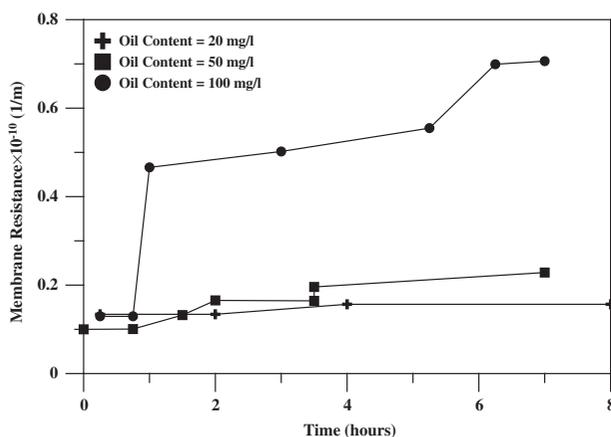
Fig. 8. Membrane resistance vs. time at permeate flux of  $40 \text{ l/m}^2 \text{ h}$ .
