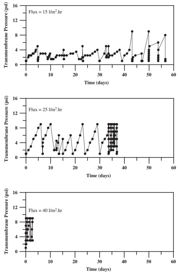
Fig. 7. TMP at different permeate flux values.
