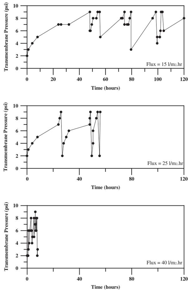
Fig. 4. TMP at oil content of 100 mg/l.
