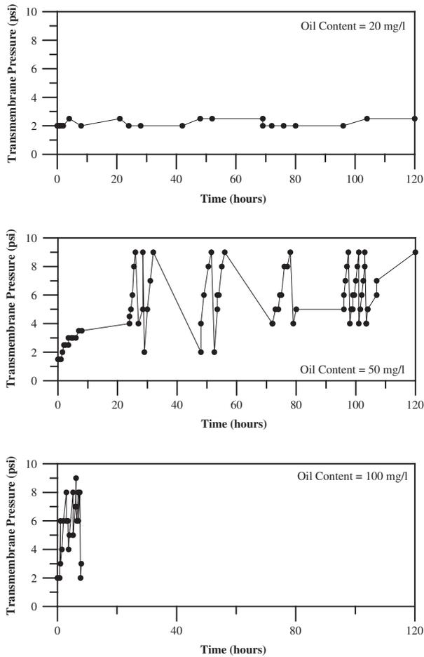
Fig. 5. TMP at permeate flux of 40 l/m<sup>2</sup> h and different oil content values.
