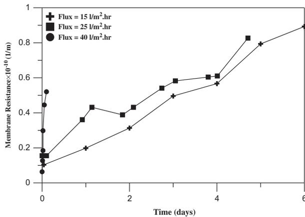
Fig. 10. Membrane resistance vs. time for field study.
