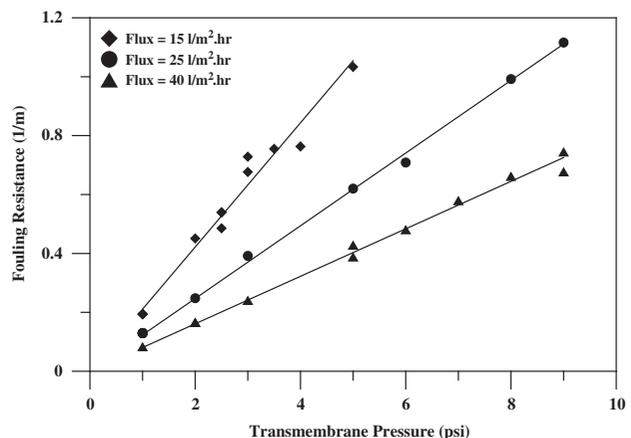
Fig. 11. Foulant resistance vs. TMP for real wastewater.
