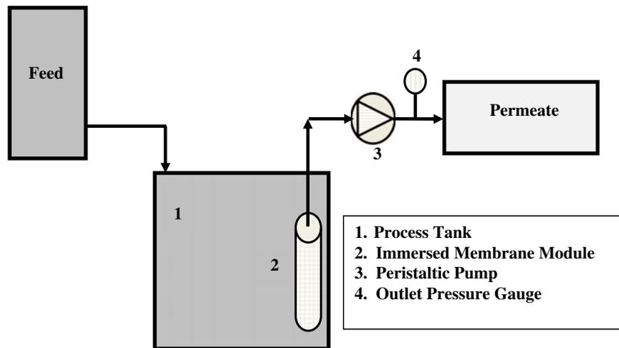
Fig. 1. Schematic diagram of the lab-scale setup.
