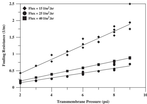
Fig. 9. Foulant resistance vs. TMP at oil content of 100 mg/l.
