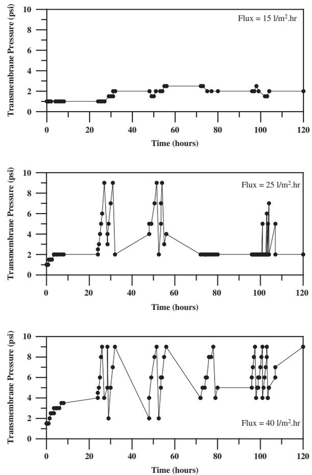
Fig. 3. TMP at oil content of  $50 \text{ mg/l}$ .
