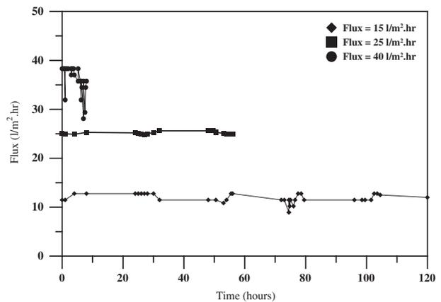
Fig. 2. Permeate flux at oil content of  $100 \text{ mg/l}$ .
