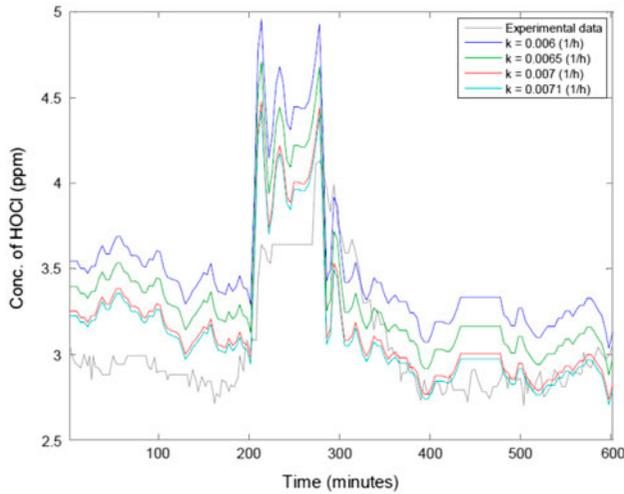
Fig. 5. Comparison of the simulated response of the model with the experimental measurements.  $k_{\text{Disinfection}} = 0.006 \text{ h}^{-1}$ ,  $k_{\text{Disinfection}} = 0.0065 \text{ h}^{-1}$ ,  $k_{\text{Disinfection}} = 0.007 \text{ h}^{-1}$ ,  $k_{\text{Disinfection}} = 0.0071 \text{ h}^{-1}$ .
