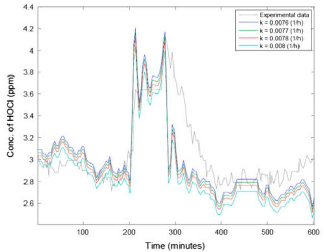
Fig. 7. Comparison of the simulated response of the model with the experimental measurements.  $k_{\text{Disinfection}} = 0.0076 \text{ h}^{-1}$ ,  $k_{\text{Disinfection}} = 0.0077 \text{ h}^{-1}$ ,  $k_{\text{Disinfection}} = 0.0078 \text{ h}^{-1}$ ,  $k_{\text{Disinfection}} = 0.008 \text{ h}^{-1}$ .
