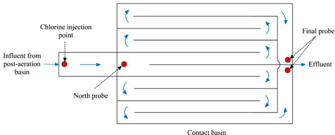
Fig. 1. Sampling points for the chlorine disinfection contact basin at the KWRF.
