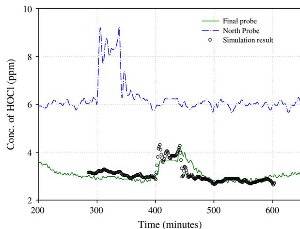
Fig. 4. Comparison of the simulation results with experimental measurements for  $k_{\text{Disinfection}} = 0.0074 \text{ h}^{-1}$ .
