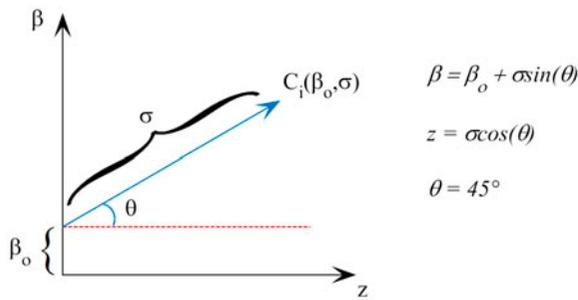
Fig. 3. Graphical representation of the odometric transformation.
