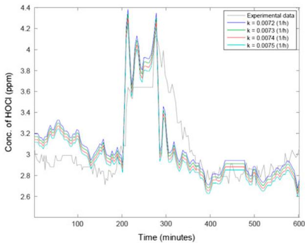
Fig. 6. Comparison of the simulated response of the model with the experimental measurements.  $k_{\text{Disinfection}} = 0.0072 \text{ h}^{-1}$ ,  $k_{\text{Disinfection}} = 0.0073 \text{ h}^{-1}$ ,  $k_{\text{Disinfection}} = 0.0074 \text{ h}^{-1}$ ,  $k_{\text{Disinfection}} = 0.0075 \text{ h}^{-1}$ .
