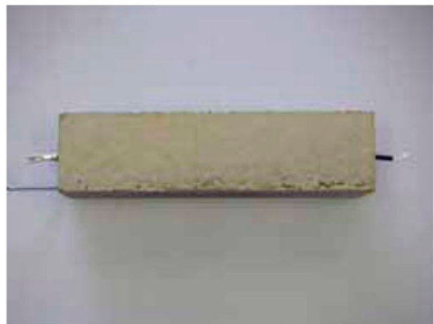
Fig. 2. Piezoelectric cable sensor mounted in concrete beam [16].
