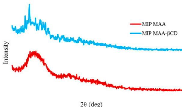
Fig. 4. X-ray diffractogram of MIP MAA- $\beta$ CD and MIP MAA.
