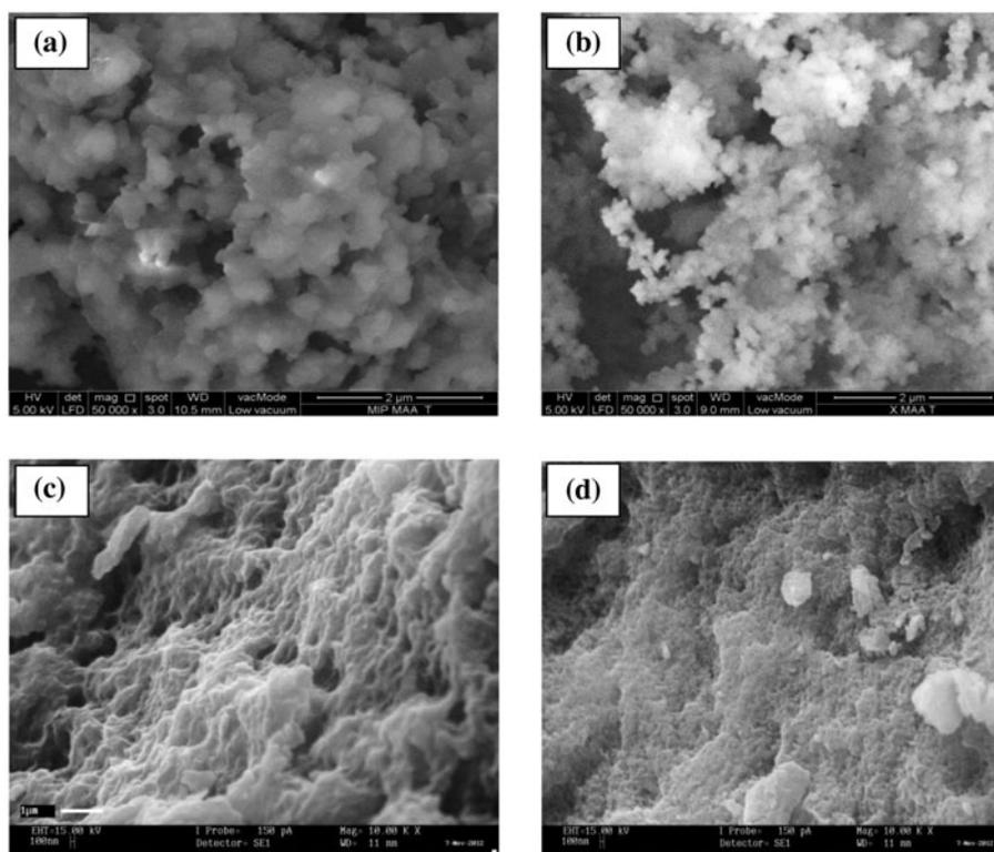
Fig. 3. SEM micrographs of the imprinted particles prepared from monomer MAA (a) MIP MAA, (b) NIP MAA and monomer MAA- $\beta$ CD, (c) MIP MAA- $\beta$ CD, and (d) NIP MAA- $\beta$ CD using cross-linker, TRIM.
