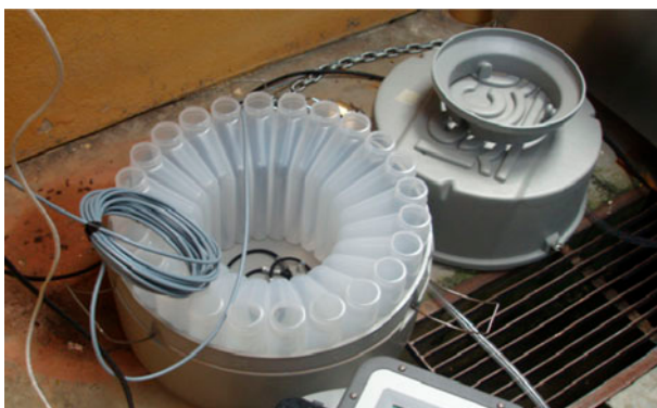
Fig. 3. 3,700 standard’s sequential base section with 24 wide-mouth, W edge-shaped Polypropylene Bottles with a Capacity of 1,000 ml Each.
