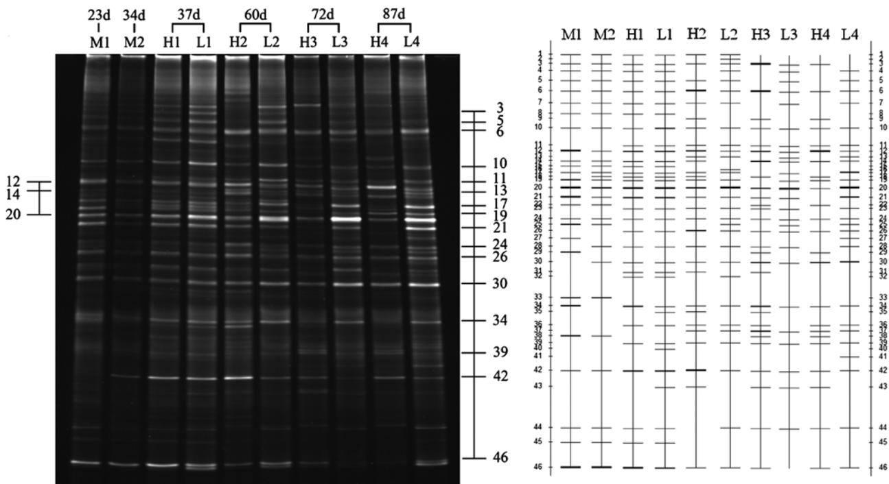
Fig. 3. DGGE profiles of samples collected from both reactors: H: high temperature (25°C); M: medium temperature (20°C); L: low temperature (15°C).
