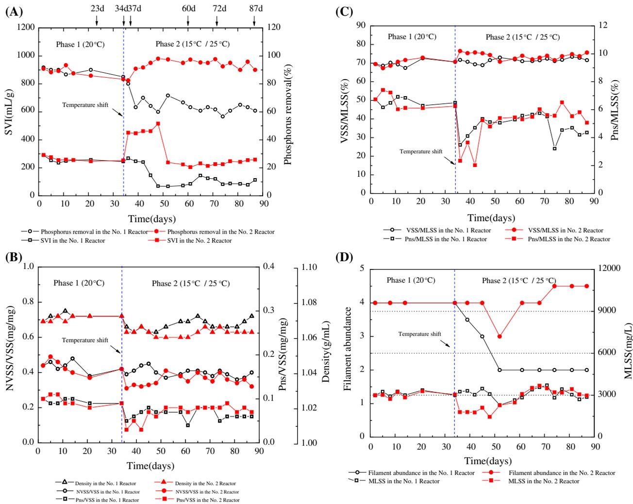
Fig. 1. Effect of temperature on sludge properties in the No. 1 and No. 2 Reactors. The arrows and numbers above the figure indicate the days when the sludge samples were collected to analyze the bacterial community structure. The blue lines show the day when the temperature in both reactors was changed. In phase 1, both reactors were operated at 20°C; in phase 2, the No. 1 and No. 2 Reactors were operated at 25 and 15°C, respectively.
