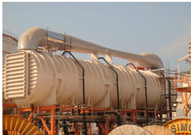
Fig. 5. MED–TVC system in Kavian petrochemical company, Iran ( http://www.fanniroo.com ).
