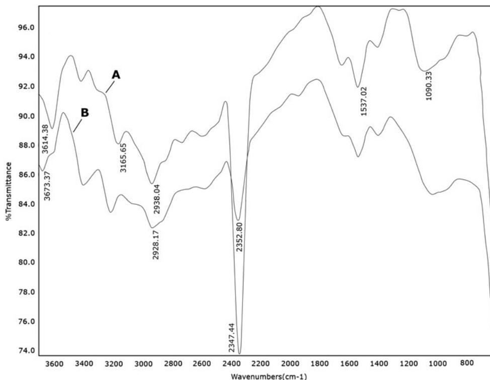
Fig. 1. FTIR Scan of waste derived tire char: (A) without dye adsorption and (B) with dye adsorption.
