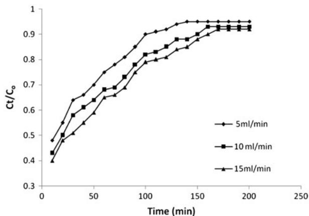
Fig. 3. Effect of flow rate on breakthrough curve for dye adsorption on WTDC (dye conc. 0.3 g/L, pH 2, bed height 10 inches).
