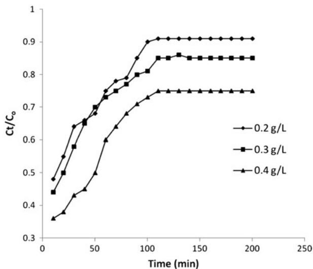
Fig. 2. Effect of initial dye concentration on breakthrough curve for dye adsorption on WTDC (bed height 10 inches, pH 2, flow rate 5 mL/min).
