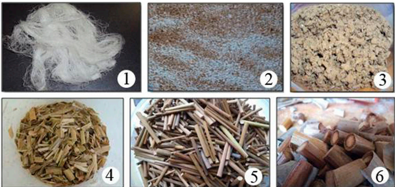
Fig. 2. Materials used as filter mediums: 1—Fibroil; 2—Duck; 3—Reo-dry; 4—reed stems ( Phragmites australis ); 5—bulrush stems ( Schoenoplectus lacustris ); 6—lesser bulrush stems ( Typha angustifolia ).
