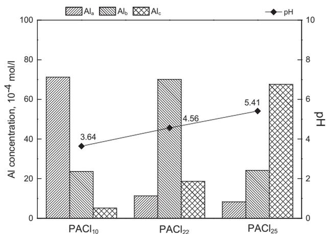
Fig. 3. Aluminum speciation and pH of  $PACl_{10}$ ,  $PACl_{22}$ , and  $PACl_{25}$ .
