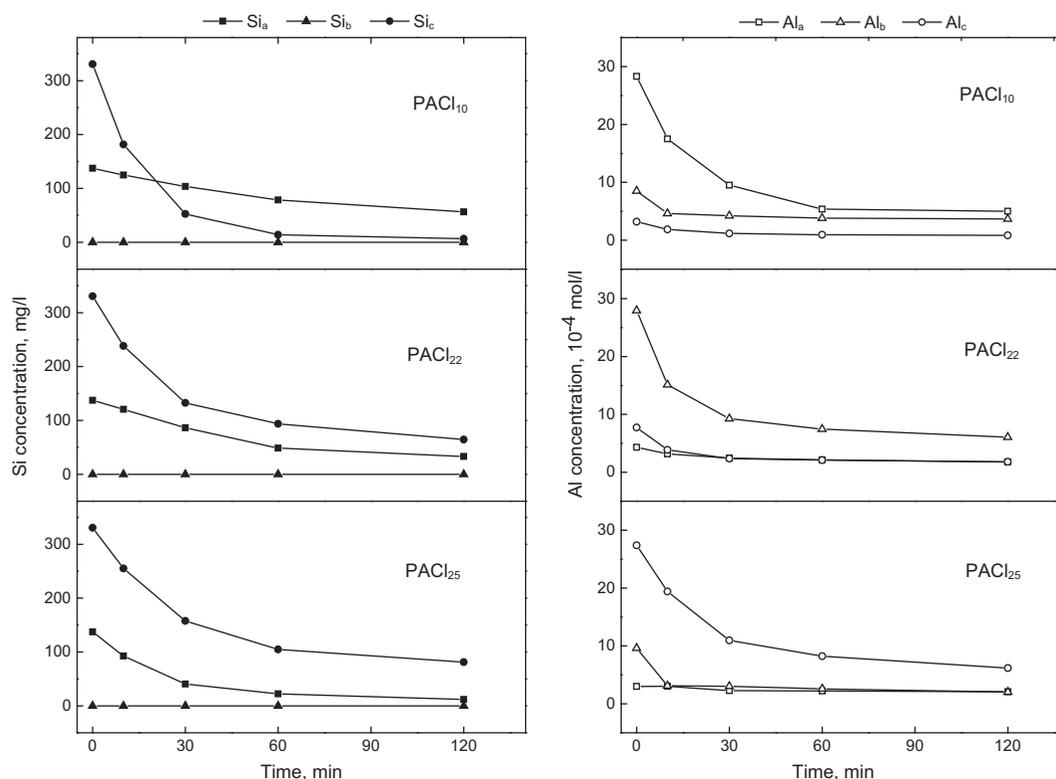
Fig. 4. Variation of silica and aluminum hydrolysates during coagulation with PACl<sub>10</sub>, PACl<sub>22</sub>, and PACl<sub>25</sub>.
