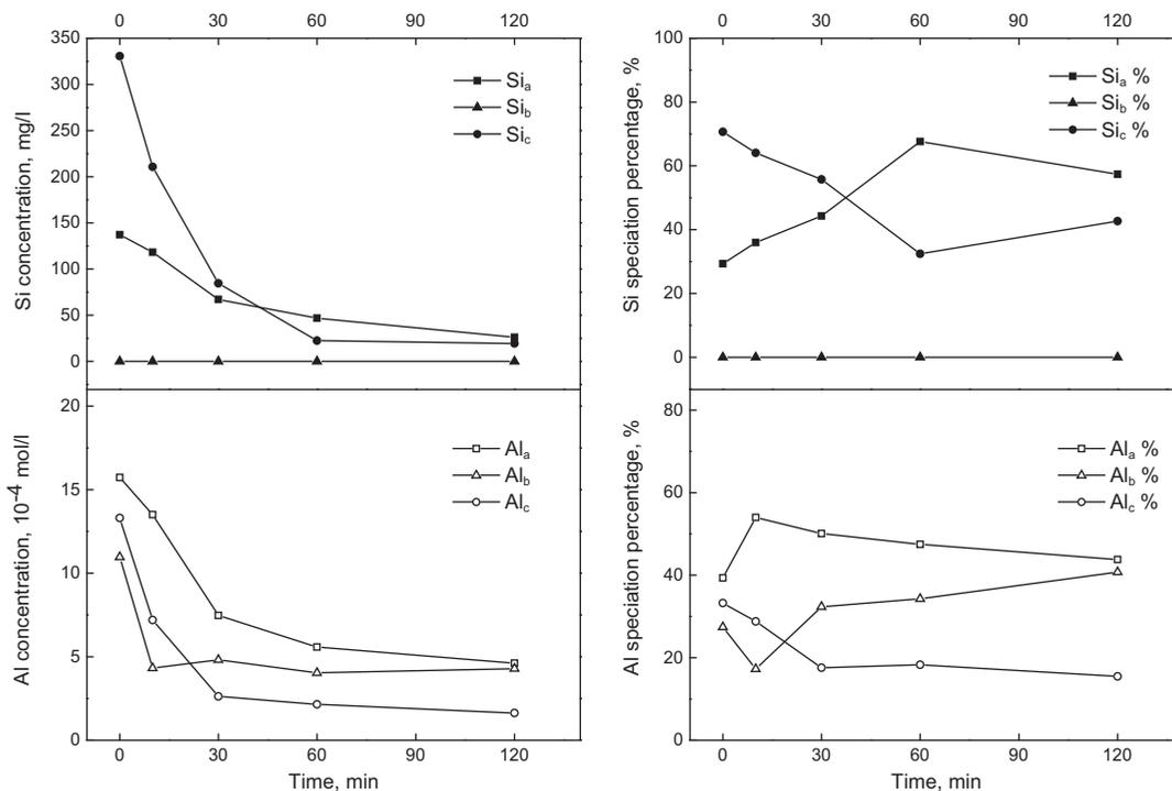
Fig. 2. Variation of silica and aluminum hydrolysates during coagulation with commercial PACI.
