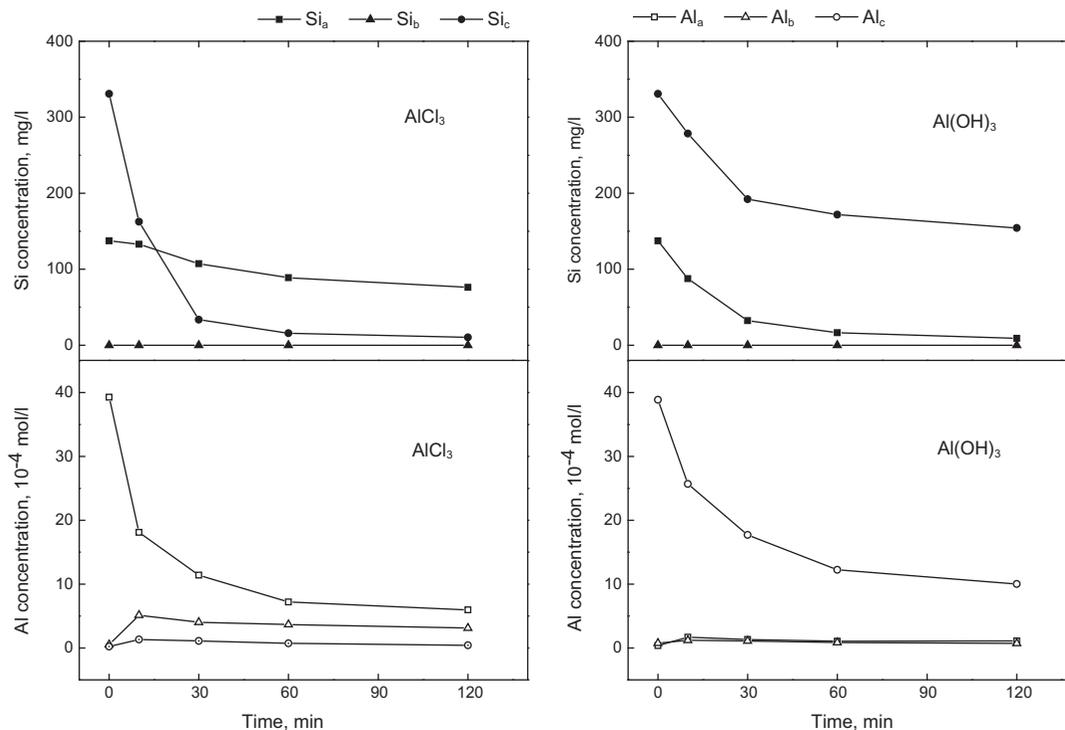
Fig. 5. Variation of silica and aluminum hydrolysate concentrations during coagulation with aluminum chloride and with amorphous aluminum hydroxide.
