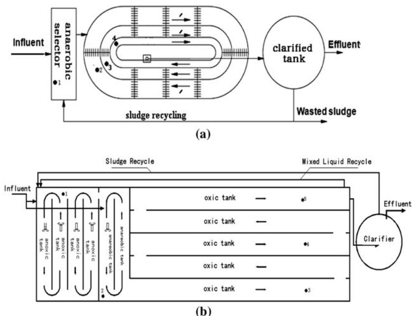
Fig. 1. Plan drawings of the two BNR processes and location of the sample points: (a) the Orbal oxidation ditch process and (b) the reversed A/A/O process.
