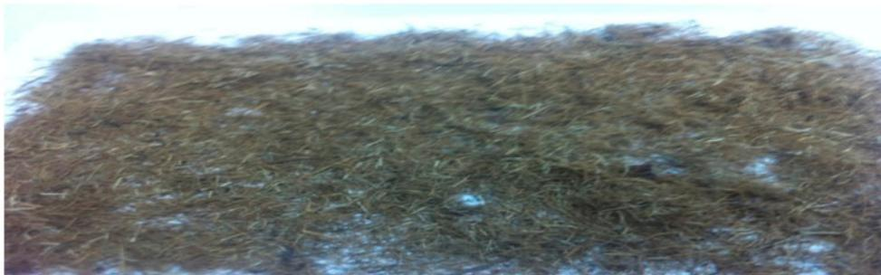
Fig. 1. Date palm fiber after drying and cutting.
