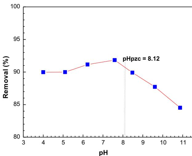
Fig. 5. Effect of initial pH on adsorption of SDBS onto ZnMgNiAl- $\text{CO}_3$  sample.
