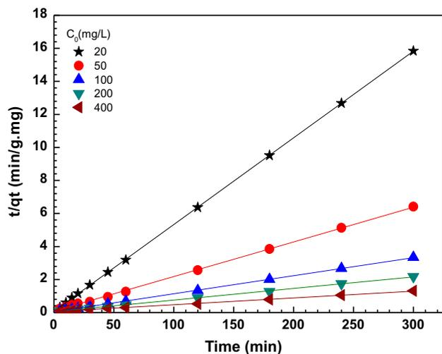
Fig. 7. Pseudo-second-order kinetic plot for the adsorption of SDBS onto ZnMgNiAl-CO<sub>3</sub>.
