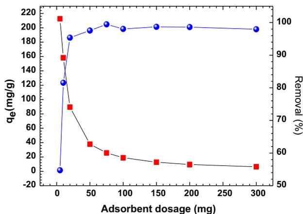
Fig. 4. Effect of the adsorbent dosage on the adsorption of SDBS onto ZnMgNiAl- $\text{CO}_3$ .
