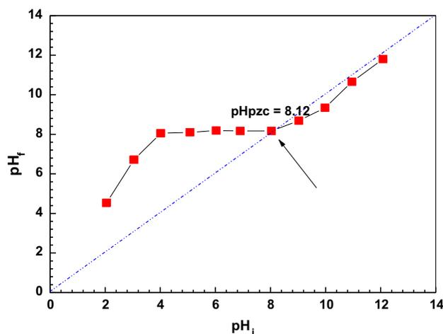
Fig. 1. Point of zero charge of ZnMgNiAl- $\text{CO}_3$ .
