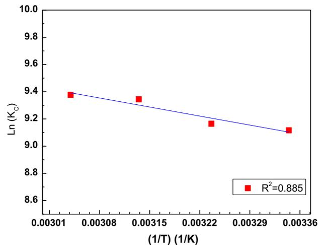
Fig. 10. Van't Hoff plot for the adsorption of SDBS onto ZnMgNiAl-CO<sub>3</sub>.
