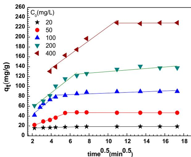
Fig. 8. The Weber-Morris plot of the kinetic data for SDBS adsorption onto ZnMgNiAl-CO<sub>3</sub> at different concentrations.
