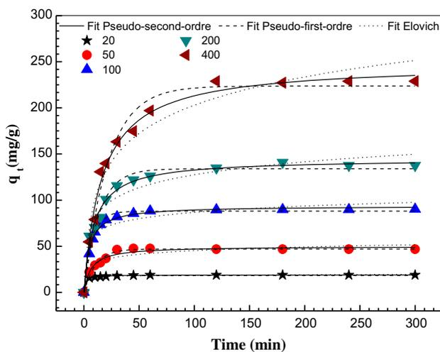
Fig. 6. Effect of contact time and initial SDBS concentrations.
