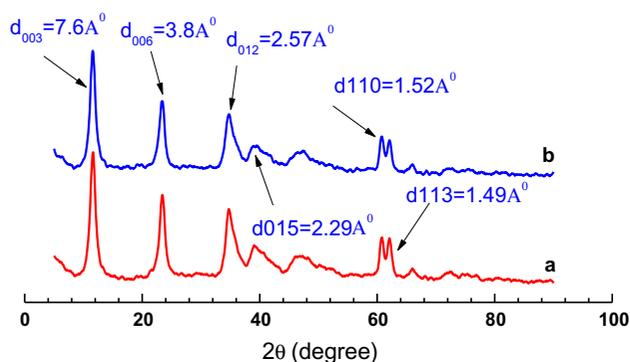
Fig. 2. Powder X-ray patterns for (a) ZnMgNi-CO<sub>3</sub> and (b) ZnMgNiAl-CO<sub>3</sub>-SDBS.
