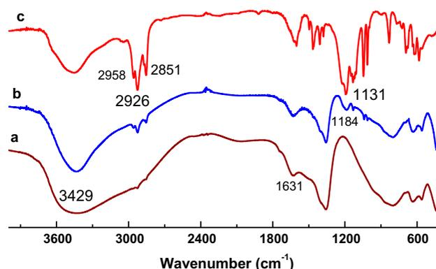
Fig. 3. FTIR spectra for (a) ZnMgNiAl-CO<sub>3</sub>, (b) ZnMgNiAl-CO<sub>3</sub>-SDBS, and (c) SDBS.
