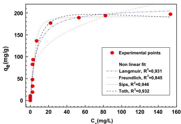
Fig. 9. SDBS adsorption isotherm onto ZnMgNiAl-CO<sub>3</sub>.
